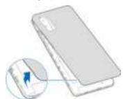
Insert the nano-SIM card into the right card slot, and insert the microSDXC card (optional) into the left card slot.
