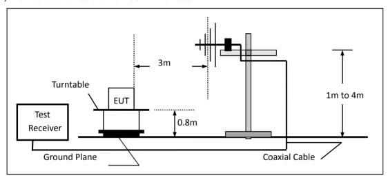
(c) For radiated emissions above 1000MHz
