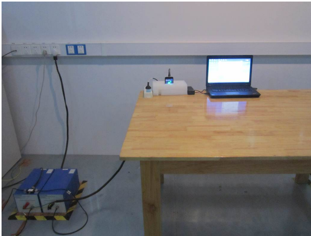
Conducted Emissions Test Setup Front View
