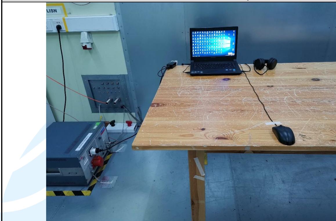
Conducted Emission Test Setup
