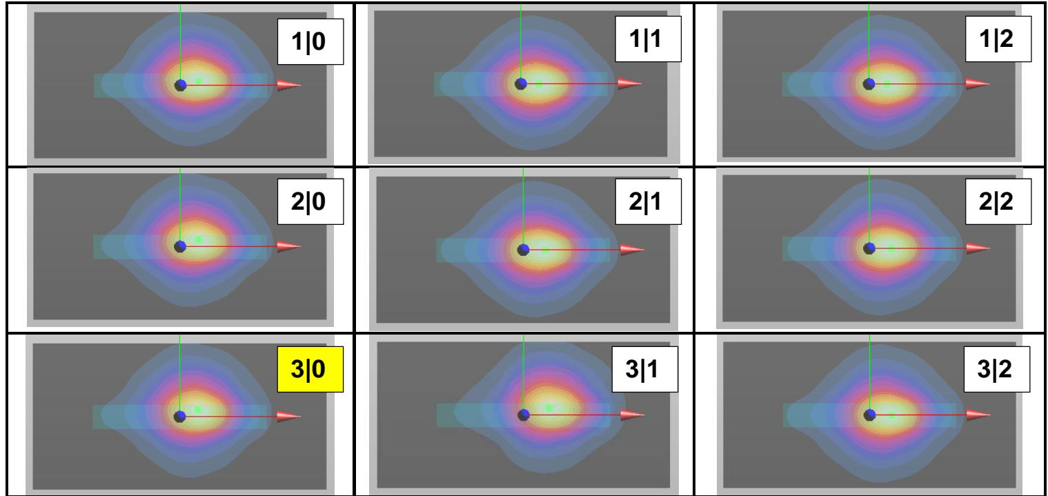
LTE2500 (Band 7) Wireless Router – Left edge facing phantom pre-screening measurement plots (10mm)
