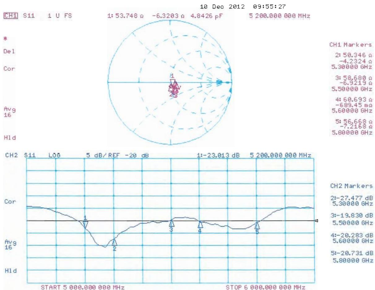
**Dipole D5000V2 – SN:1048 Antenna Parameters measured: 2014-04-07.**
