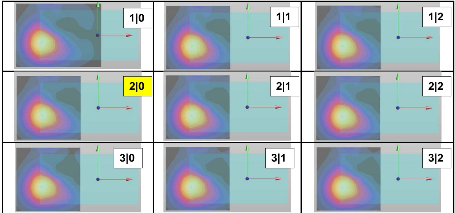
LTE2500 (Band 7) Body – Display facing phantom SAR pre-screening measurement plots (15mm)
