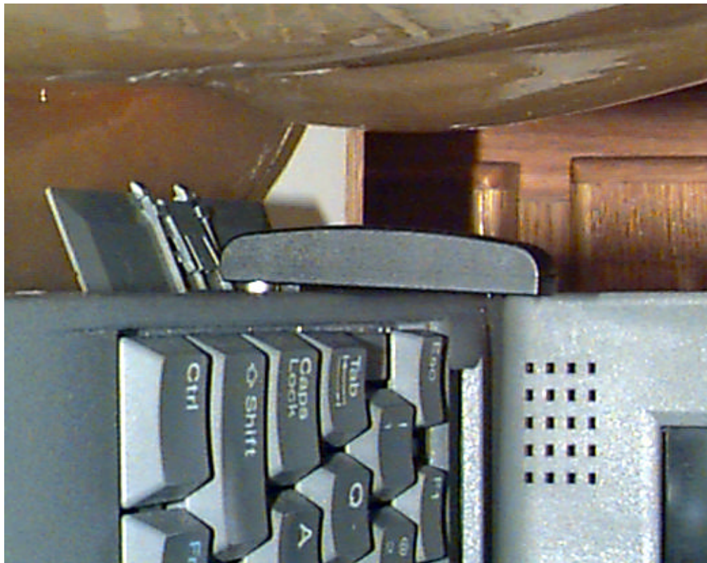
Figure 8. Test setup of EUT in normal operating position with the source of significant emissions (antenna) 2.0 cm below the phantom.
