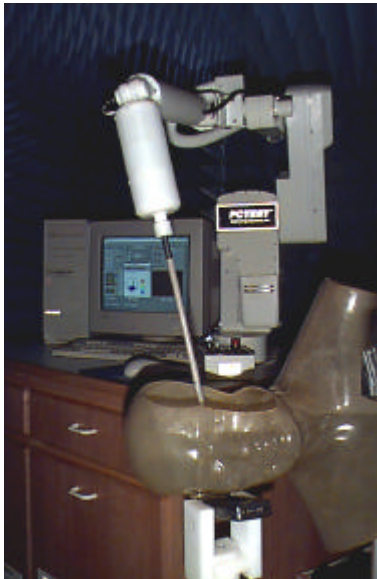
Figure 5. Photograph of the Probe and the Phantom
