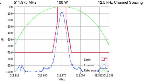
DMR 511.9750MHz Mask D 100W RBW=100Hz, VBW=1000Hz, Detector Mode=Peak Result=Pass
