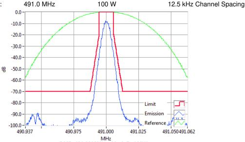
DMR 491.0000MHz Mask D 100W RBW=100Hz, VBW=1000Hz, Detector Mode=Peak Result=Pass
