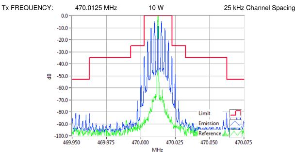
Analogue Modulation 470.0125MHz Mask B 10W RBW=300Hz, VBW=3000Hz, Detector Mode=Peak Result=Pass
