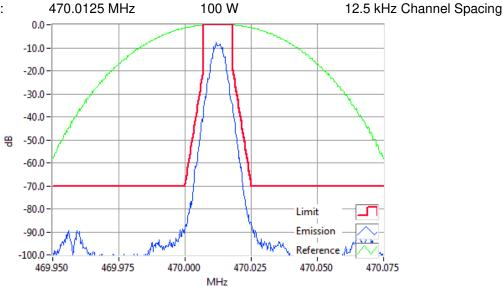
DMR 470.0125MHz Mask D 100W RBW=100Hz, VBW=1000Hz, Detector Mode=Peak Result=Pass
