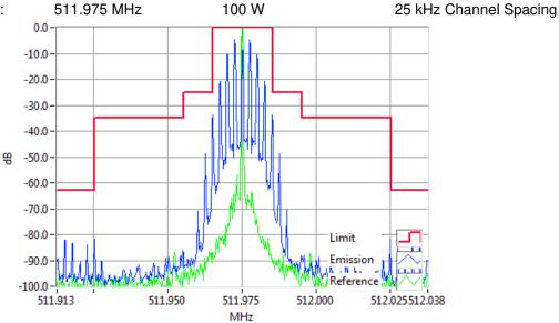
Analogue Modulation 511.9750MHz Mask B 100W RBW=300Hz, VBW=3000Hz, Detector Mode=Peak Result=Pass
