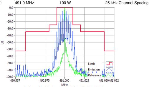
Analogue Modulation 491.0000MHz Mask B 100W RBW=300Hz, VBW=3000Hz, Detector Mode=Peak Result=Pass
