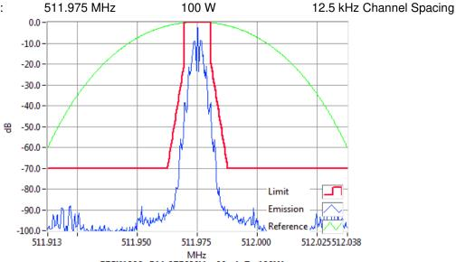
FFSK1200 511.9750MHz Mask D 100W RBW=100Hz, VBW=1000Hz, Detector Mode=Peak Result=Pass
