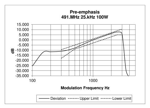
SPECIFICATION: FCC CFR 2.1047 (a)
