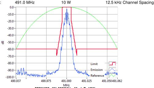
FFSK1200 491.0000MHz Mask D 10W RBW=100Hz, VBW=1000Hz, Detector Mode=Peak Result=Pass
