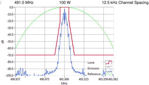
FFSK1200 491.0000MHz Mask D 100W RBW=100Hz, VBW=1000Hz, Detector Mode=Peak Result=Pass
