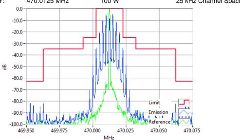
Analogue Modulation 470.0125MHz Mask B 100W RBW=300Hz, VBW=3000Hz, Detector Mode=Peak Result=Pass
