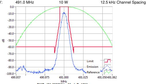
DMR 491.0000MHz Mask D 10W RBW=100Hz, VBW=1000Hz, Detector Mode=Peak Result=Pass
