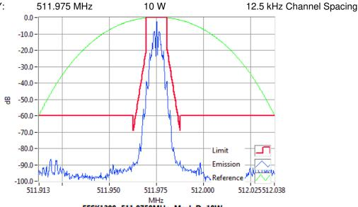
FFSK1200 511.9750MHz Mask D 10W RBW=100Hz, VBW=1000Hz, Detector Mode=Peak Result=Pass
