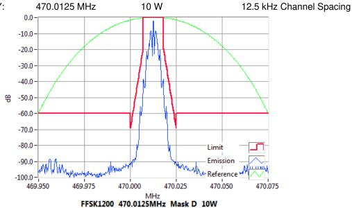
RBW=100Hz, VBW=1000Hz, Detector Mode=Peak Result=Pass
