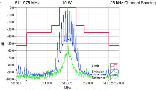
Analogue Modulation 511.9750MHz Mask B 10W RBW=300Hz, VBW=3000Hz, Detector Mode=Peak Result=Pass
