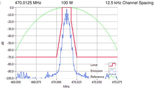
FFSK1200 470.0125MHz Mask D 100W RBW=100Hz, VBW=1000Hz, Detector Mode=Peak Result=Pass
