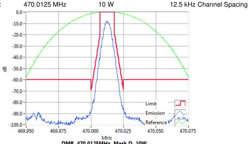
DMR 470.0125MHz Mask D 10W RBW=100Hz, VBW=1000Hz, Detector Mode=Peak Result=Pass
