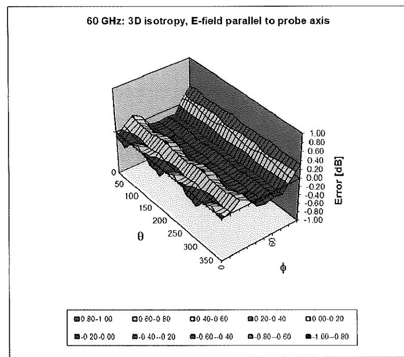
Probe isotropy for  $E_{\text{tot}}$ : probe rotated  $\phi = 0^\circ$  to  $360^\circ$ , tilted from field propagation direction  $\vec{k}$
