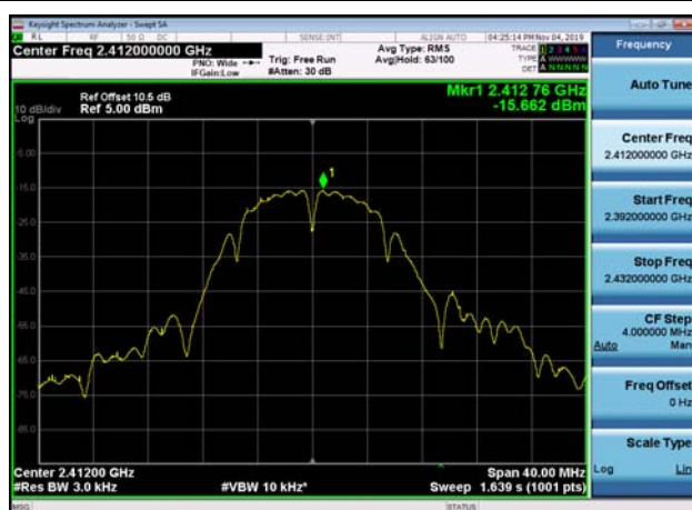
Power spectral density-802.11b ,2462MHz
