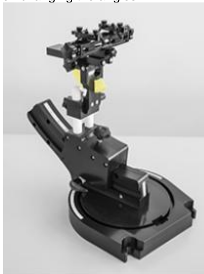
Device holder supplied by SPEAG
