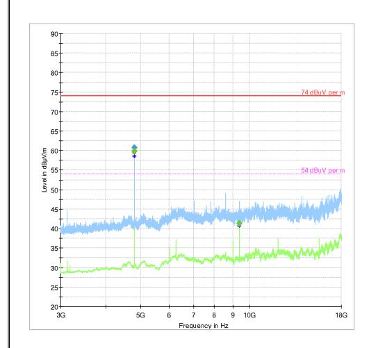
Note: According to FCC15.35(c), a duty cycle correction factor is applied here. Considering the limit of packets per interval and minimum interval of BTLE, this leads a correction factor of 17.86dB. Hence this margn could cover the highest spurious above.
