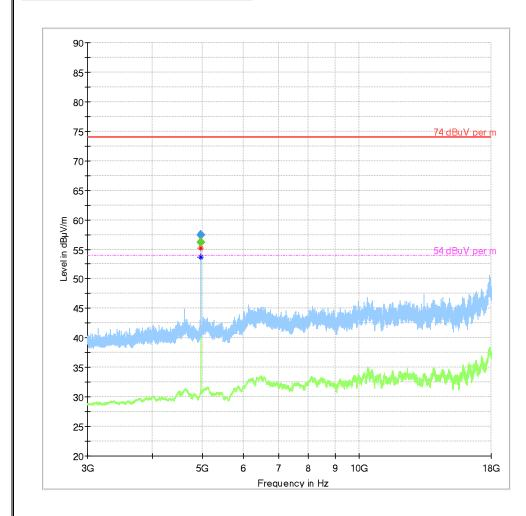
Note: According to FCC15.35(c), a duty cycle correction factor is applied here. Considering the limit of packets per interval and minimum interval of BTLE, this leads a correction factor of 17.86dB. Hence this margn could cover the highest spurious above.
