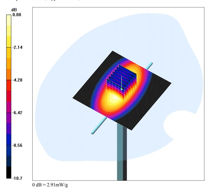
Communication System: CW; Frequency: 900 MHz; Duty Cycle: 1:1
