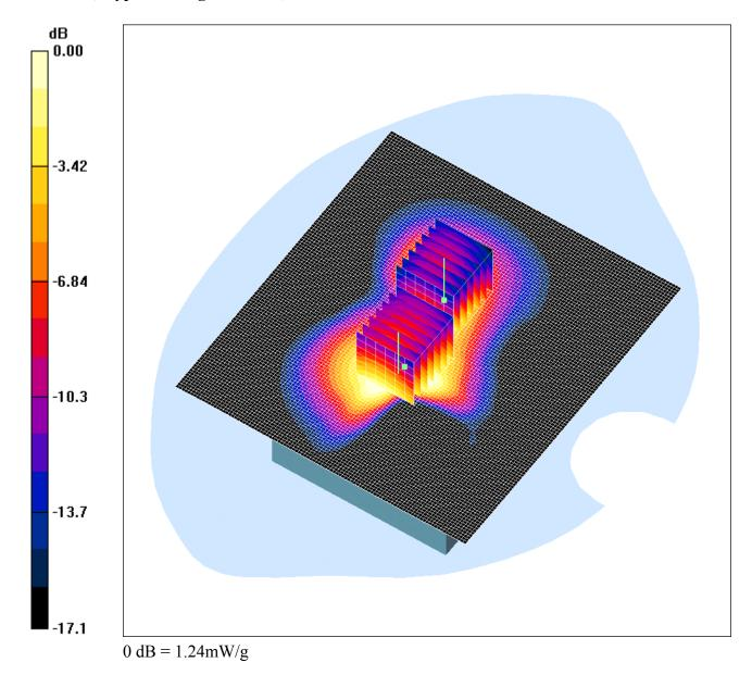
Communication System: DCS 1900; Frequency: 1879.8 MHz; Duty Cycle: 1:8.3
