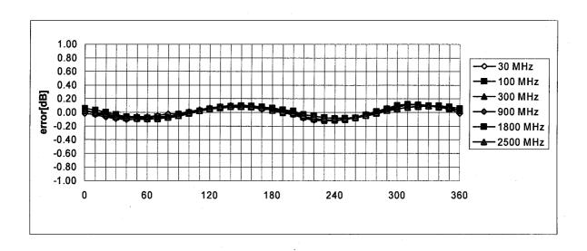
Axial Isotropy Error  $< \pm 0.2 \text{ dB}$
