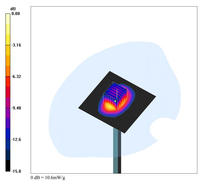
Communication System: CW; Frequency: 1800 MHz; Duty Cycle: 1:1
