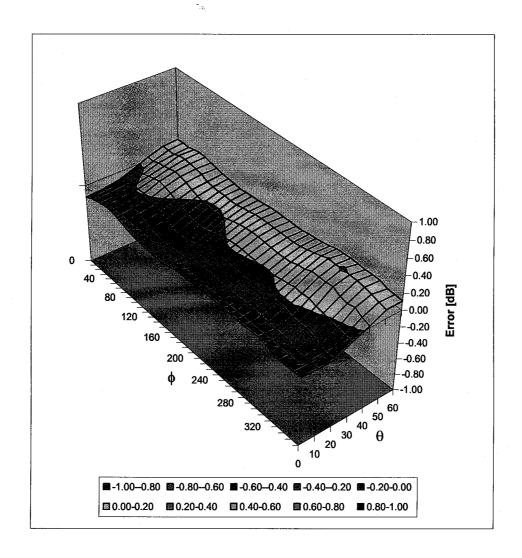
Spherical Isotropy Error < ± 0.4 dB
