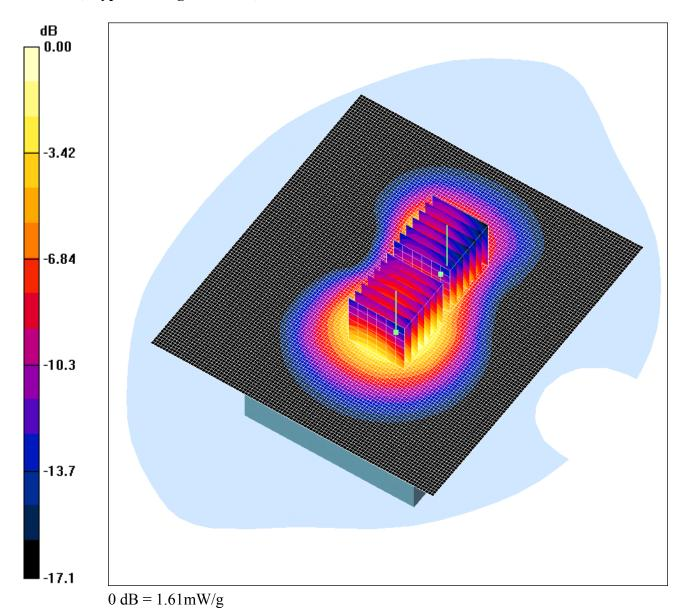
Communication System: DCS 1900; Frequency: 1850.2 MHz; Duty Cycle: 1:8.3
