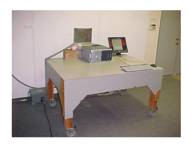
AC Conducted Emissions Measurement (Front View) Setup
