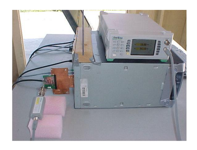
Maximum Peak Output Power Measurement Setup
