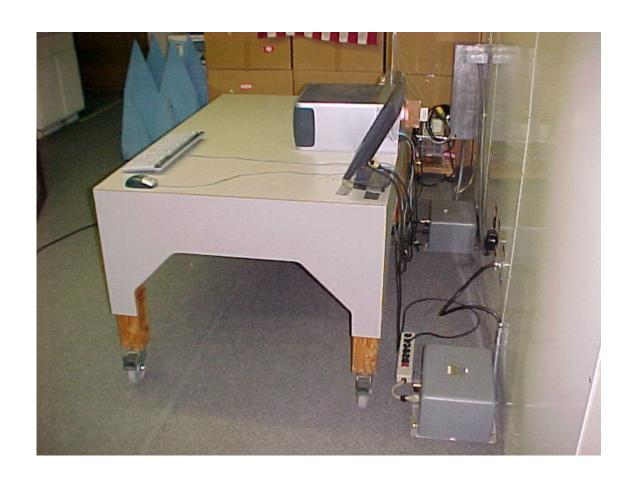
AC Conducted Emissions Measurement (Rear View) Setup
