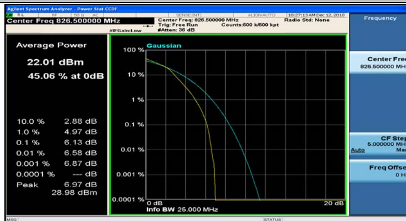
(Channel Bandwidth: 5 MHz)_LCH_16QAM_25RB#0
