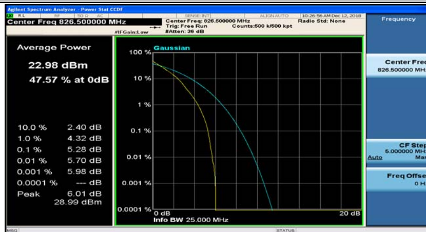
(Channel Bandwidth: 5 MHz)_LCH_QPSK_25RB#0
