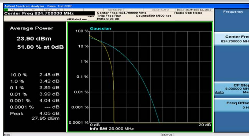
(Channel Bandwidth: 1.4 MHz)_LCH_QPSK_3RB#0
