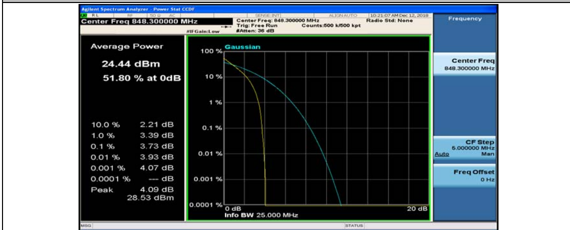
(Channel Bandwidth: 1.4 MHz)_HCH_QPSK_6RB#0
