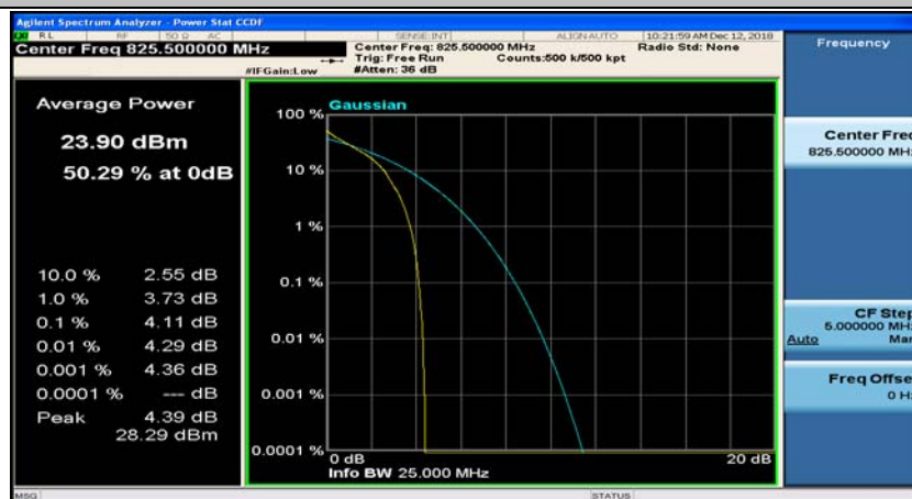
(Channel Bandwidth: 3 MHz)_LCH_QPSK_8RB#0
