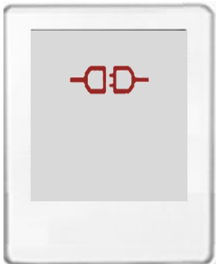
Disconnected with Gateway
