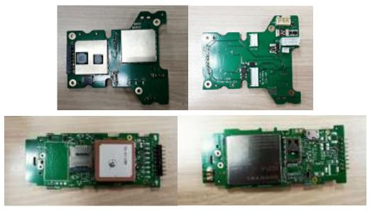
2) Complete equipment of Flex2-L. For the complete equipment, as shown below. After installation, the device sometimes connects the harness, and some will not connect the harness.
