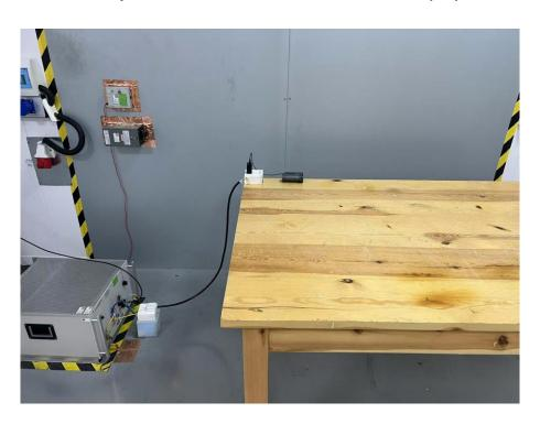
Set-up for Radiated Emission (RE), Below 1GHz
