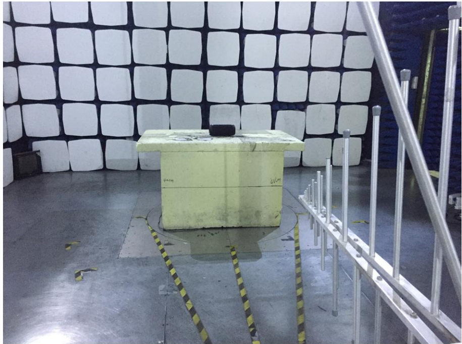
Radiation Emission Test Setup (30MHz to 1GHz)
