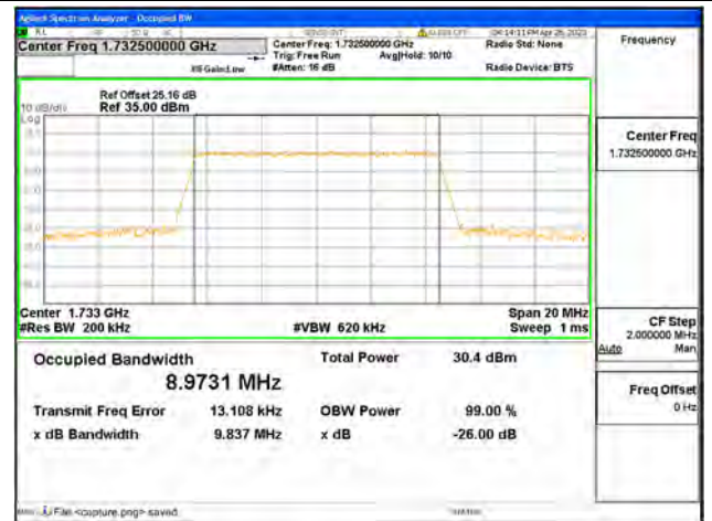
Band4 / 10MHz / 16QAM/ Mid CH
