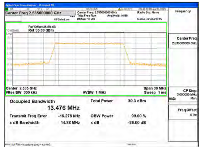
Band7 / 15MHz / 16QAM/ Mid CH
