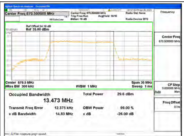
Band71 / 15MHz / 16QAM/ Low CH
