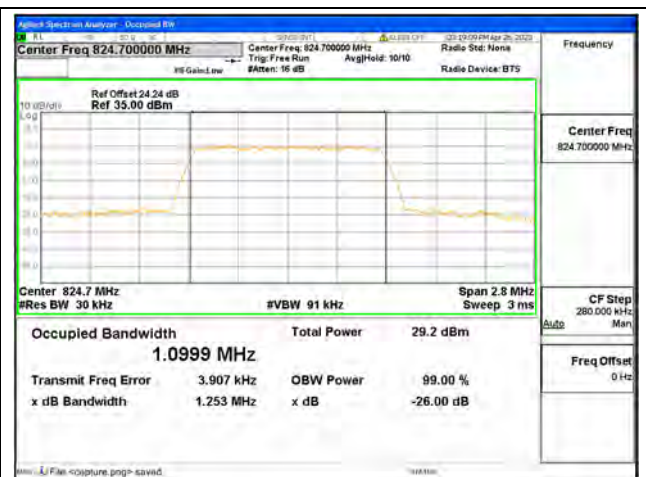
Band5 / 1.4MHz / 16QAM/ Low CH
