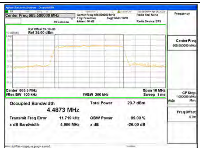
Band71 / 5MHz / 16QAM/ Low CH
