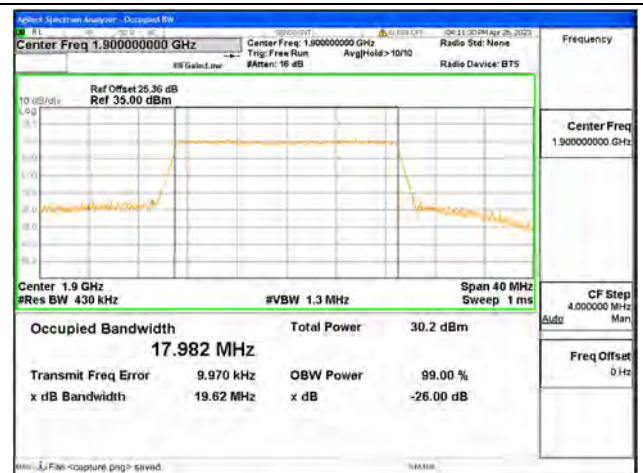
Band2 / 20MHz / 16QAM/ High CH
