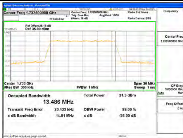
Band4 / 15MHz / QPSK/ Mid CH
