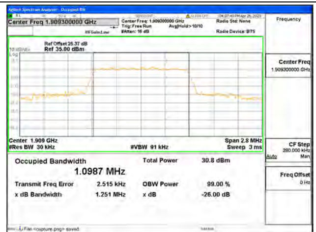
Band2 / 1.4MHz / 16QAM/ High CH
