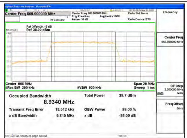
Band71 / 10MHz / 16QAM/ Low CH
