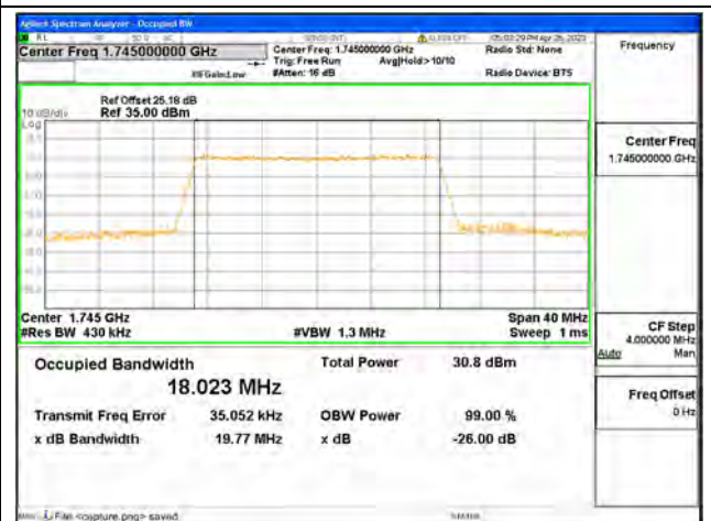
Band4 / 20MHz / 16QAM/ High CH
