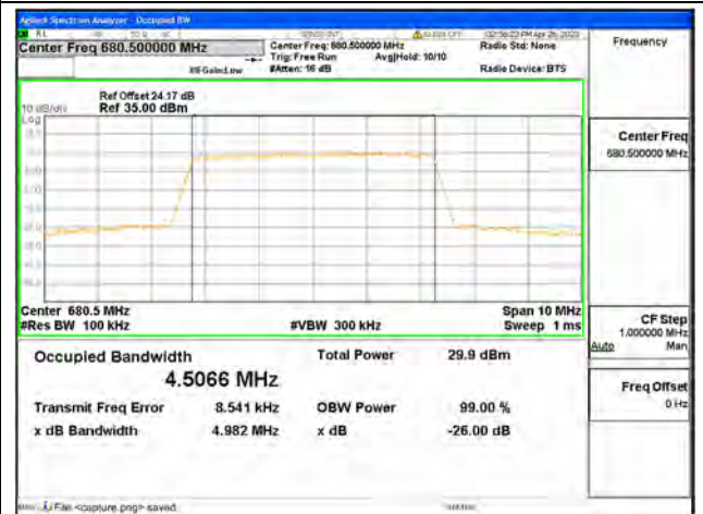
Band71 / 5MHz / 16QAM/ Mid CH
