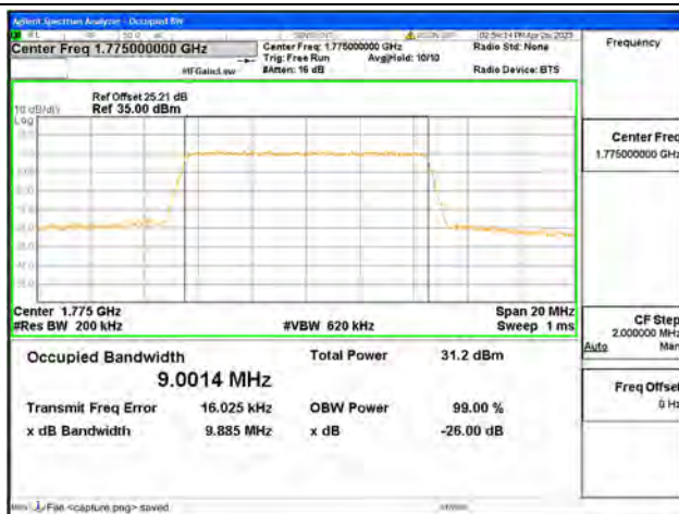
Band66 / 10MHz / QPSK/ High CH
