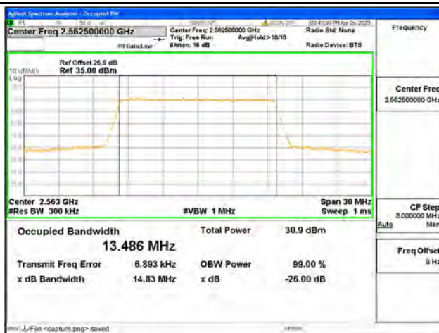
Band7 / 15MHz / QPSK/ High CH
