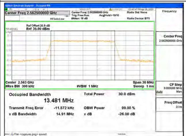
Band7 / 15MHz / 16QAM/ High CH
