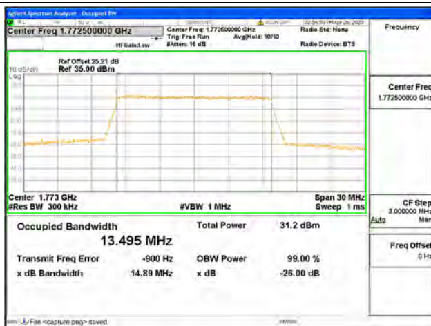
Band66 / 15MHz / QPSK/ High CH
