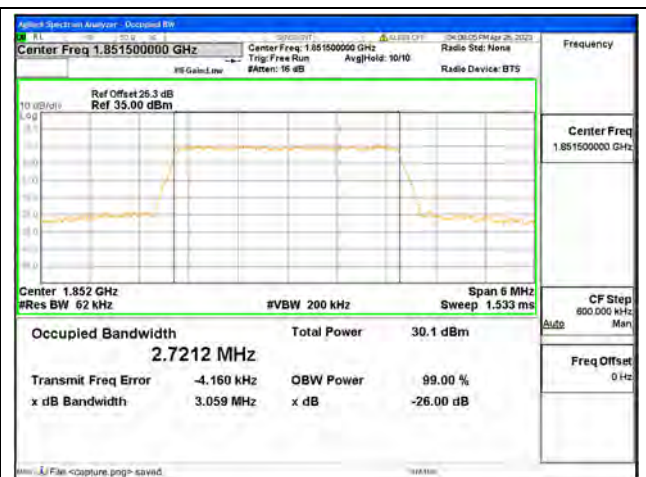
Band2 / 3MHz / 16QAM/ Low CH
