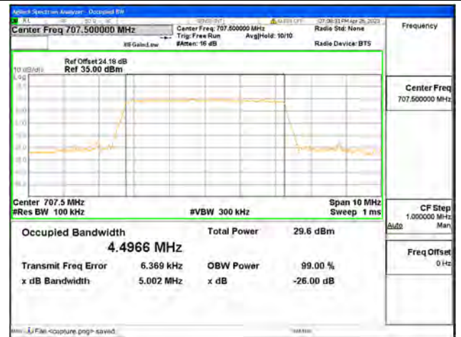
Band12 / 5MHz / 16QAM/ Mid CH
