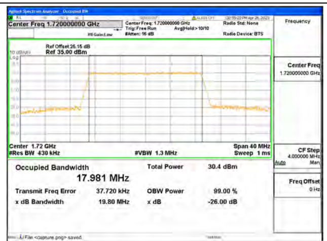
Band66 / 20MHz / 16QAM/ Low CH
