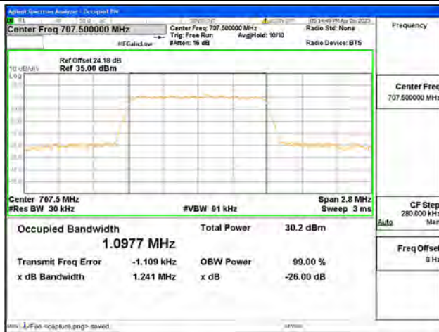
Band12 / 1.4MHz / QPSK/ Mid CH
