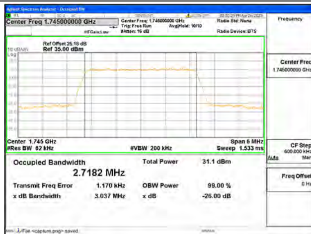
Band66 / 3MHz / QPSK/ Mid CH
