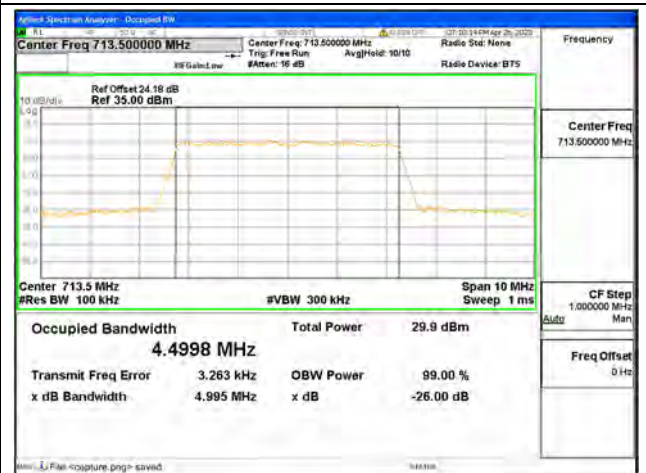
Band17 / 5MHz / 16QAM/ High CH
