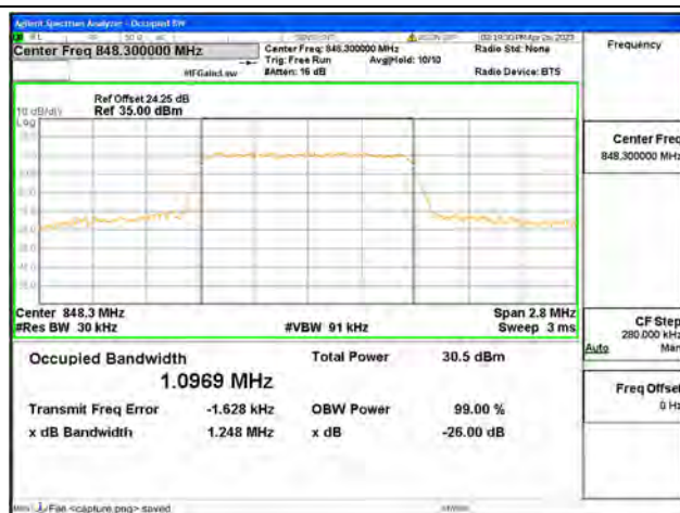
Band5 / 1.4MHz / QPSK/ High CH
