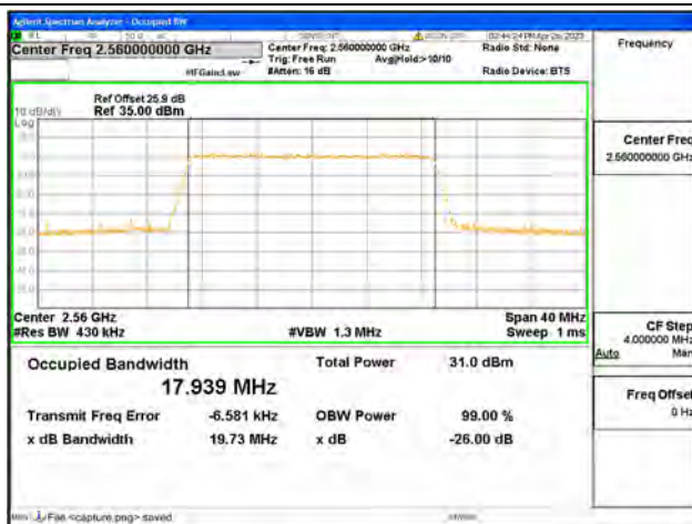
Band7 / 20MHz / QPSK/ High CH
