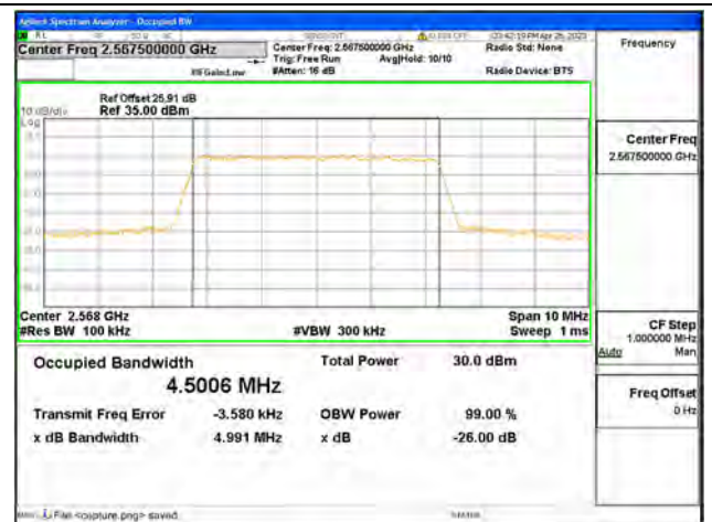
Band7 / 5MHz / 16QAM/ High CH
