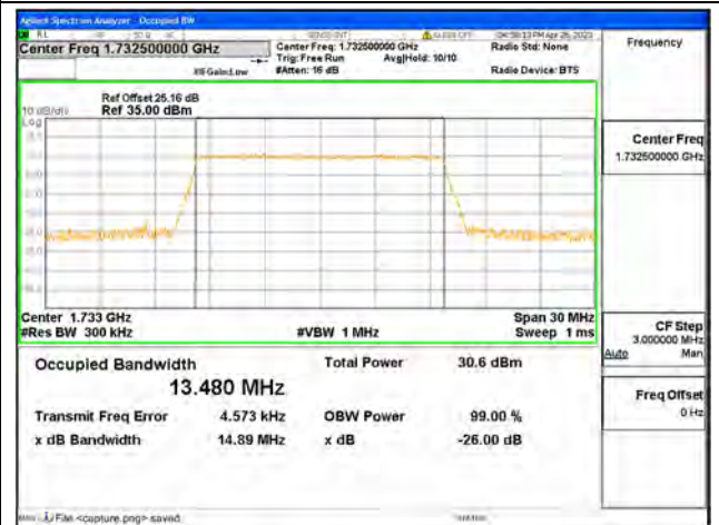
Band4 / 15MHz / 16QAM/ Mid CH
