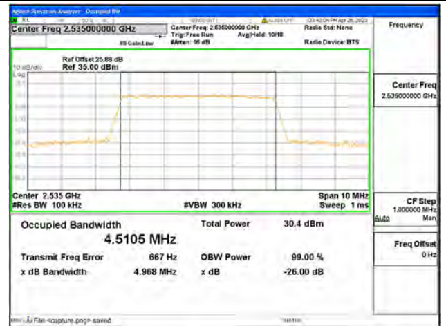
Band7 / 5MHz / 16QAM/ Mid CH
