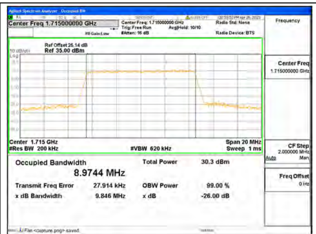
Band66 / 10MHz / 16QAM/ Low CH
