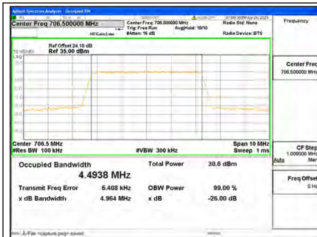
Band17 / 5MHz / QPSK/ Low CH
