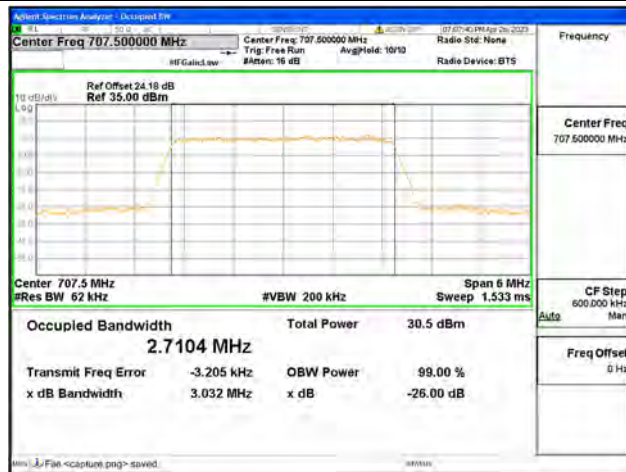
Band12 / 3MHz / QPSK/ Mid CH
