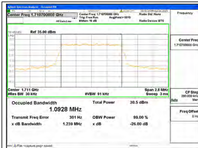
Band66 / 1.4MHz / QPSK/ Low CH
