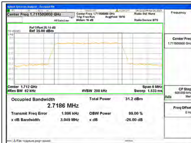
Band4 / 3MHz / QPSK/ Low CH
