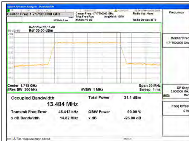
Band66 / 15MHz / QPSK/ Low CH
