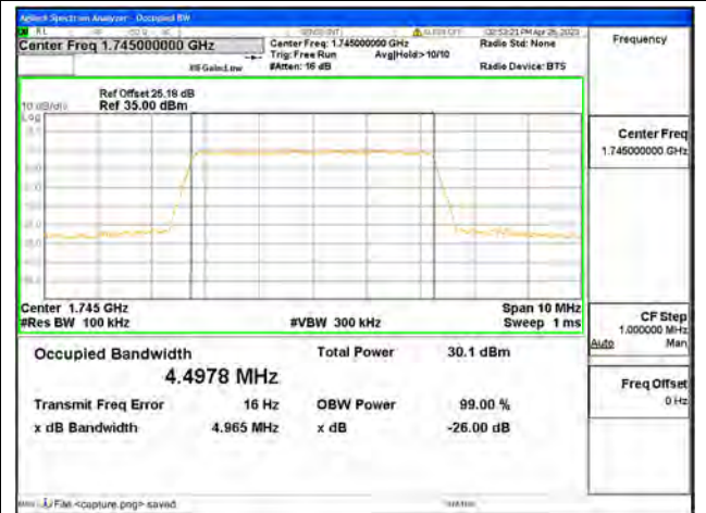
Band66 / 5MHz / 16QAM/ Mid CH
