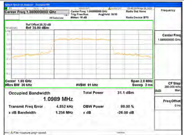
Band2 / 1.4MHz / 16QAM/ Mid CH
