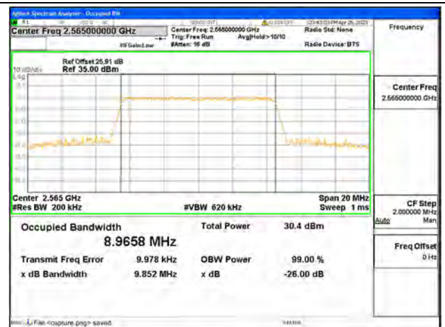
Band7 / 10MHz / 16QAM/ High CH
