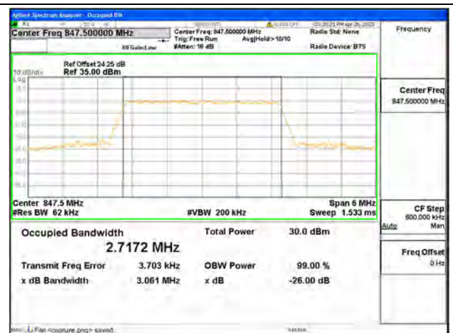
Band5 / 3MHz / 16QAM/ High CH
