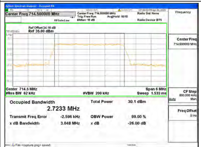
Band12 / 3MHz / 16QAM/ High CH
