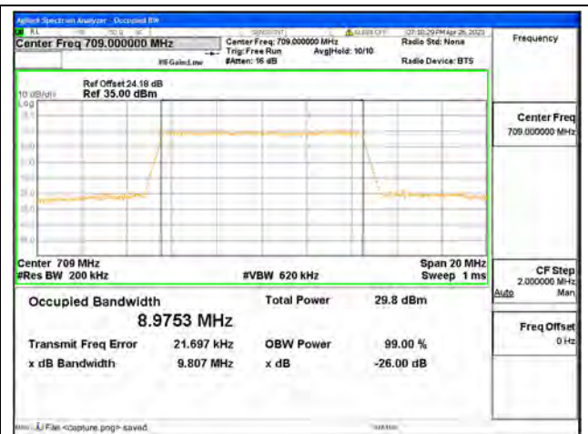
Band17 / 10MHz / 16QAM/ Low CH
