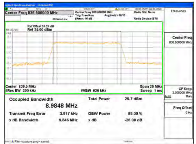
Band5 / 10MHz / 16QAM/ Mid CH
