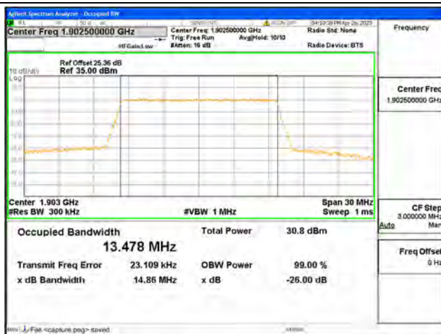
Band2 / 15MHz / QPSK/ High CH
