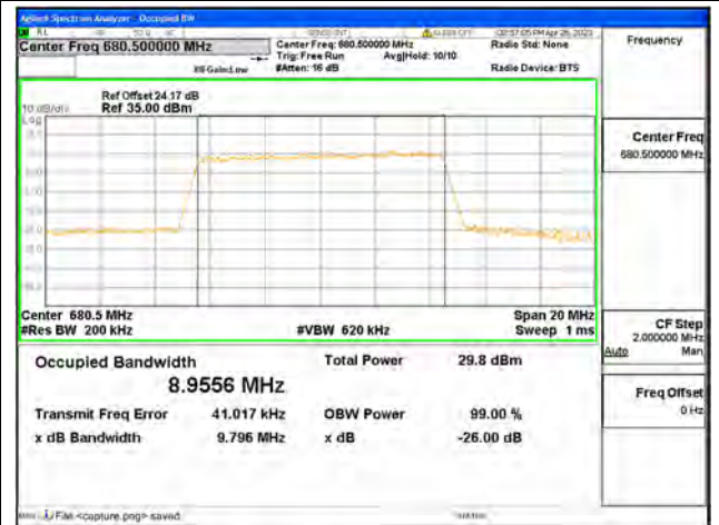
Band71 / 10MHz / 16QAM/ Mid CH
