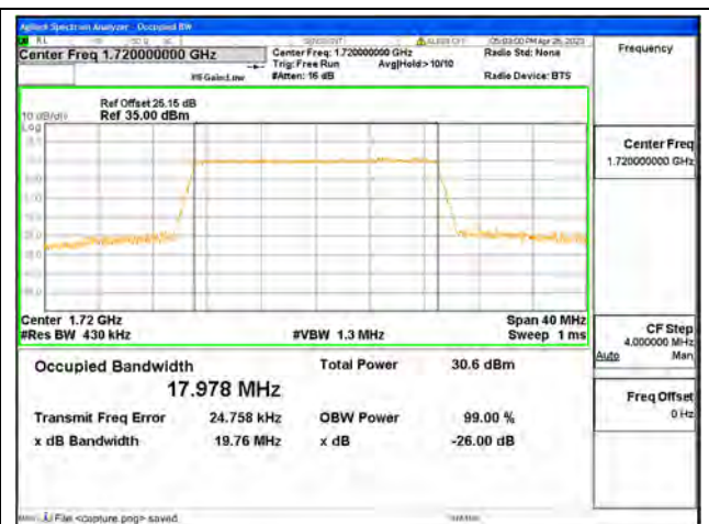
Band4 / 20MHz / 16QAM/ Low CH
