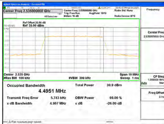
Band7 / 5MHz / QPSK/ Mid CH
