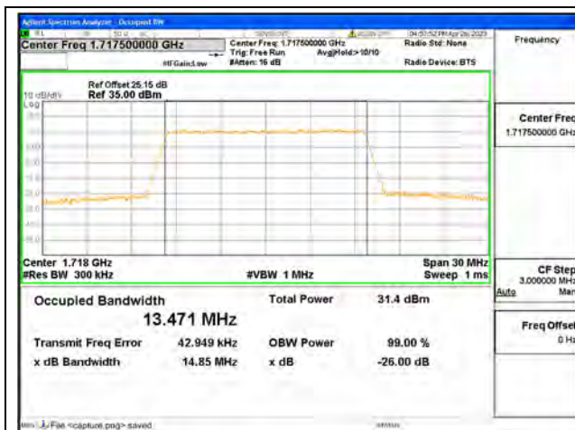
Band4 / 15MHz / QPSK/ Low CH
