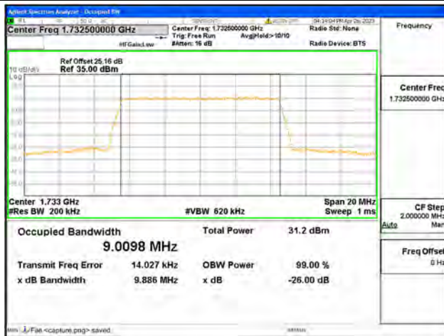
Band4 / 10MHz / QPSK/ Mid CH
