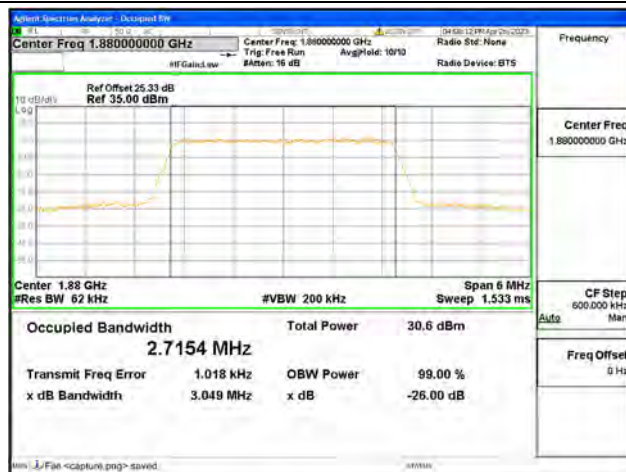
Band2 / 3MHz / QPSK/ Mid CH
