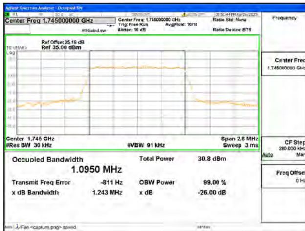
Band66 / 1.4MHz / QPSK/ Mid CH
