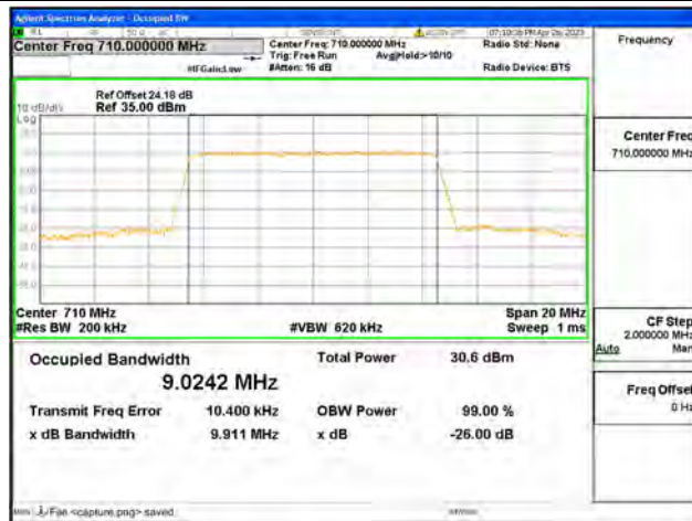
Band17 / 10MHz / QPSK/ Mid CH
