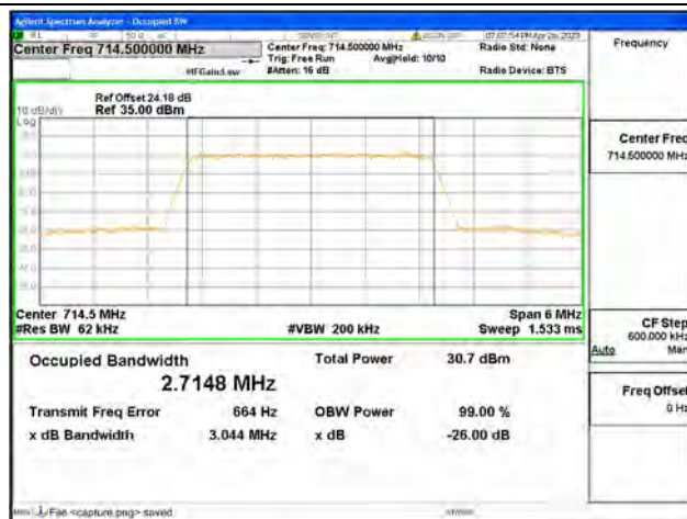
Band12 / 3MHz / QPSK/ High CH
