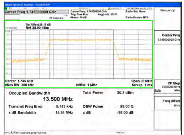
Band66 / 15MHz / 16QAM/ Mid CH
