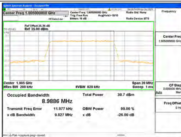
Band2 / 10MHz / QPSK/ High CH
