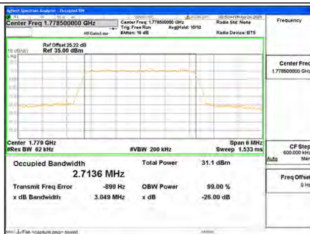
Band66 / 3MHz / QPSK/ High CH
