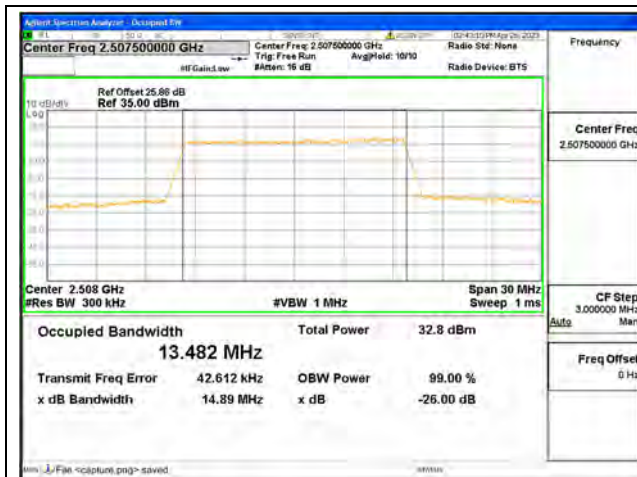
Band7 / 15MHz / QPSK/ Low CH
