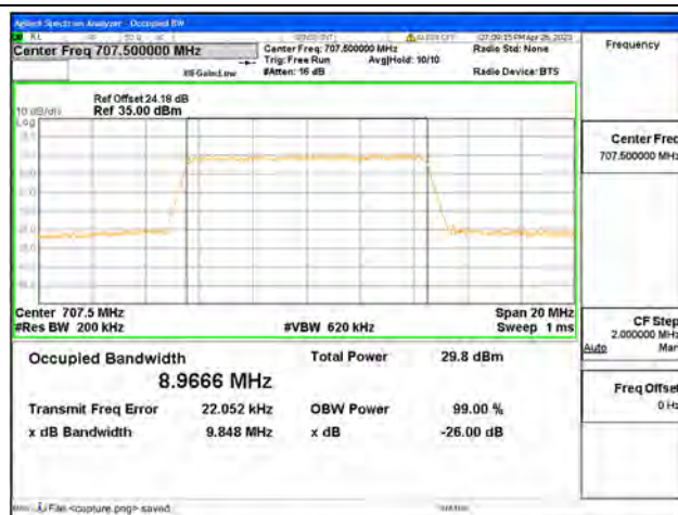
Band12 / 10MHz / 16QAM/ Mid CH
