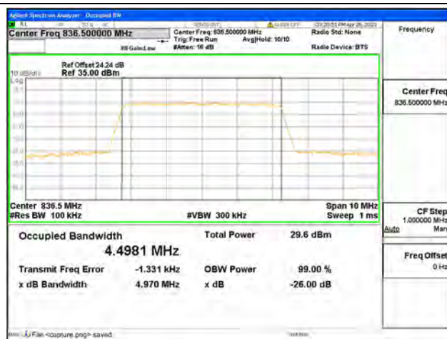
Band5 / 5MHz / 16QAM/ Mid CH
