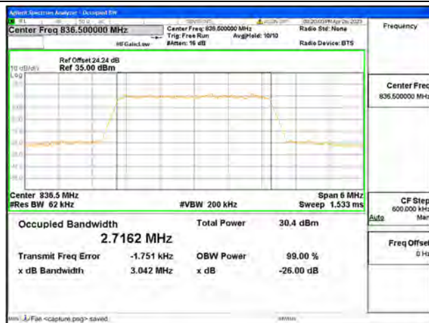
Band5 / 3MHz / QPSK/ Mid CH
