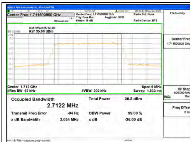
Band66 / 3MHz / QPSK/ Low CH
