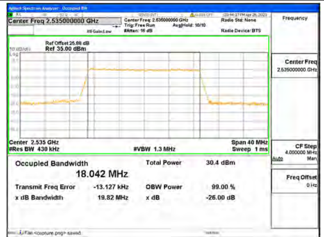
Band7 / 20MHz / 16QAM/ Mid CH
