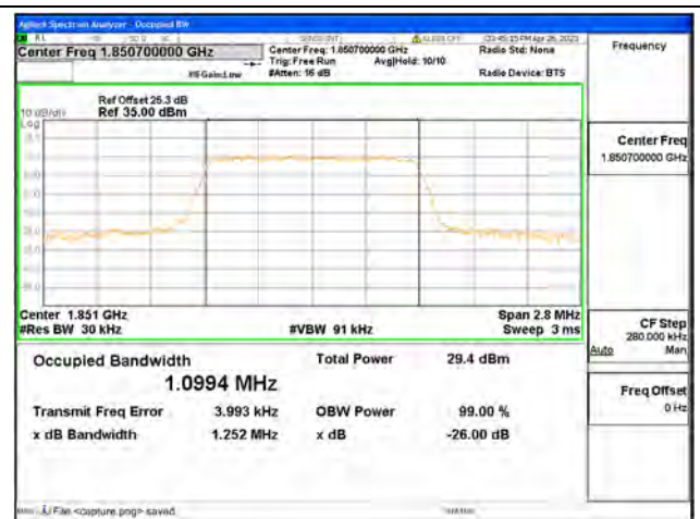
Band2 / 1.4MHz / 16QAM/ Low CH
