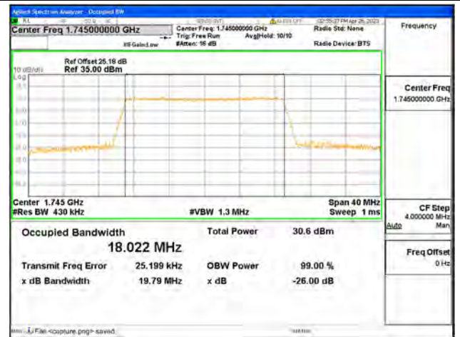
Band66 / 20MHz / 16QAM/ Mid CH
