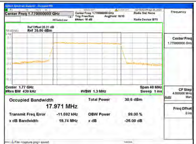
Band66 / 20MHz / 16QAM/ High CH
