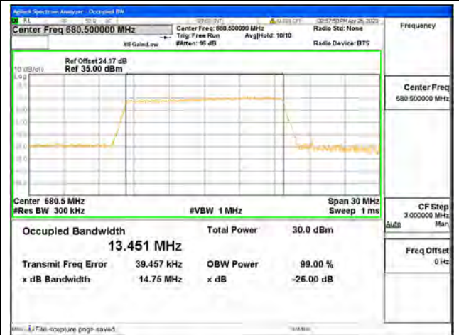
Band71 / 15MHz / 16QAM/ Mid CH
