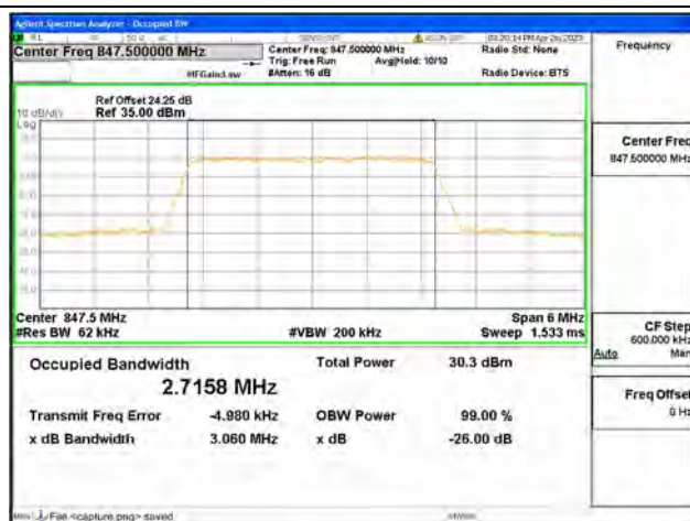
Band5 / 3MHz / QPSK/ High CH
