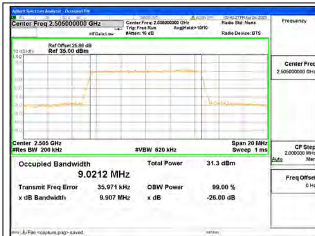
Band7 / 10MHz / QPSK/ Low CH
