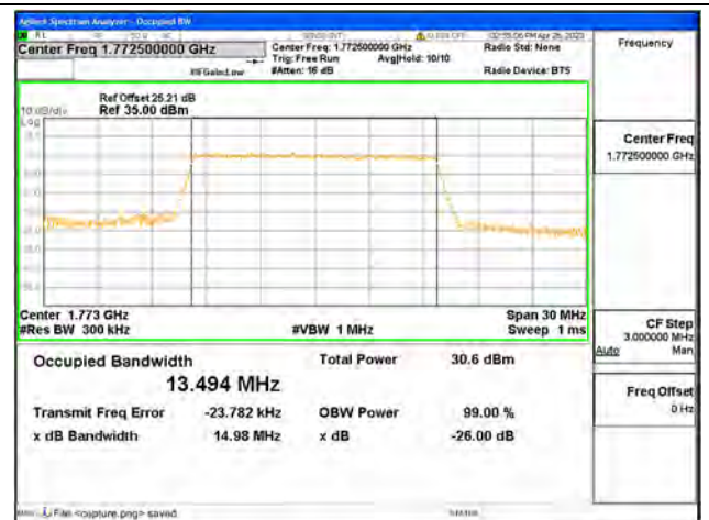
Band66 / 15MHz / 16QAM/ High CH
