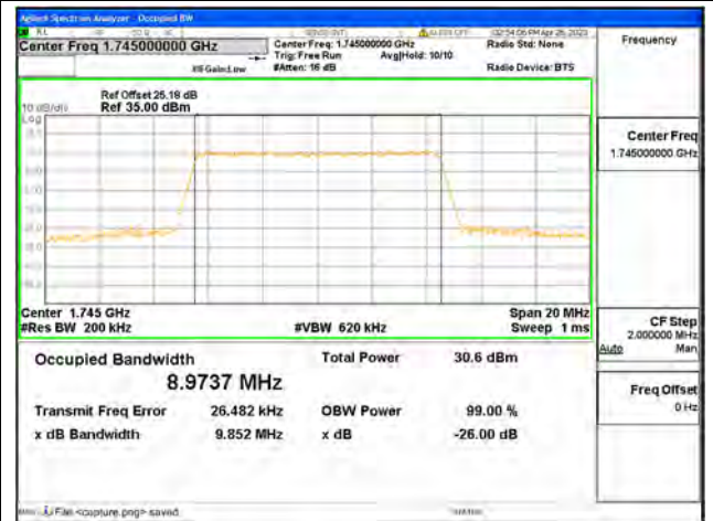
Band66 / 10MHz / 16QAM/ Mid CH
