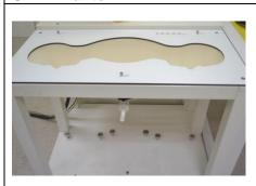
Construction: The shell corresponds to the specifications of the Specific Anthropomorphic Mannequin (SAM) phantom defined in IEEE1528: 2013. It enables the dosimetric evaluation of left and right hand phone usage as well as body mounted usage at the flat phantom region. A cover prevents evaporation of the liquid. Reference markings on the phantom allow the complete setup of all predefined phantom positions and measurement grids by manually teaching three points with the robot.
