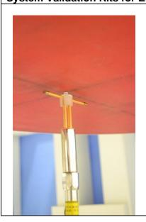
Construction: Symmetrical dipole with I/4 balun Enables
