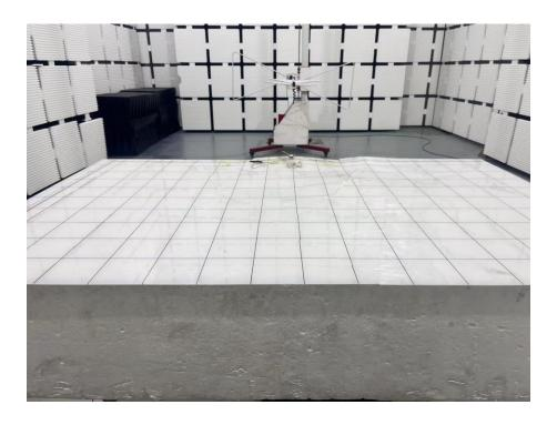
Set-up for Radiated Spurious Emission, Above 1GHz
