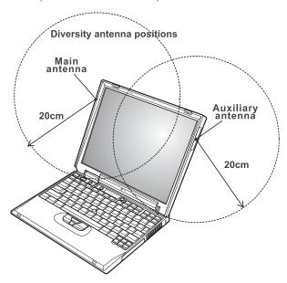
**Note:** The transmission diversity function is implemented for the Card (FCC ID: ANOU58H004). The function does not emit radio frequencies simultaneously from both antennas. One of the antennas is selected automatically or manually (by users) to have good quality of radiocommunication.
