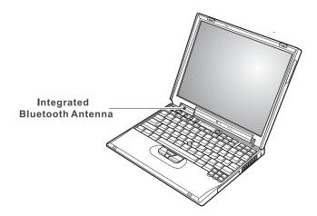
**Note:** The antenna of IBM Integrated Bluetooth with 56K Modem is located in the left hinge portion of keyboard. Transmitted energy from the Bluetooth device is very low compared to other RF devices. Therefore a 20 cm separation from the Bluetooth antenna is not required.
