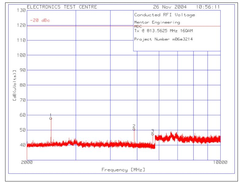
Plot of Conducted Emissions: -13 dBm = 94 dB $\mu$ V
