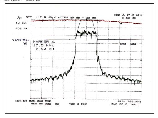
Spectrum Analyzer Plot: Emission Mask G: Tx @ 813 MHz Attenuation = 22.9 dB
