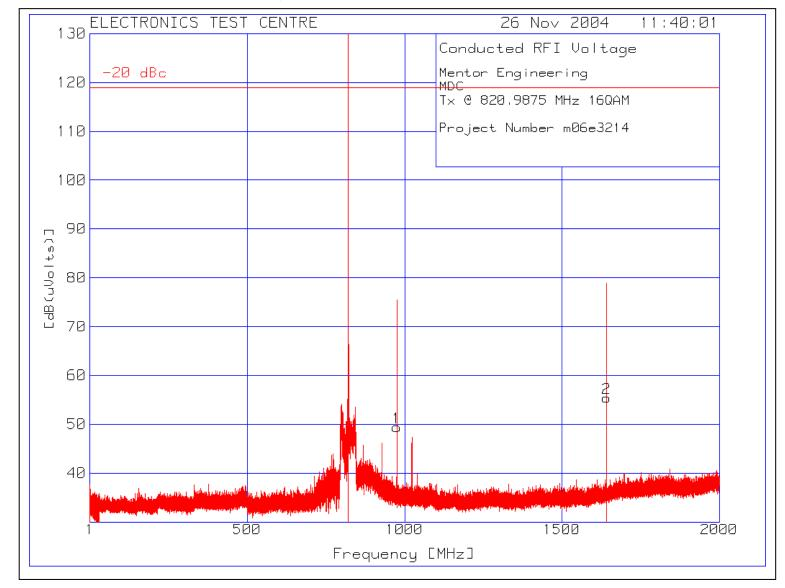
Plot of Conducted Emissions: -13 dBm = 94 dB $\mu$ V
