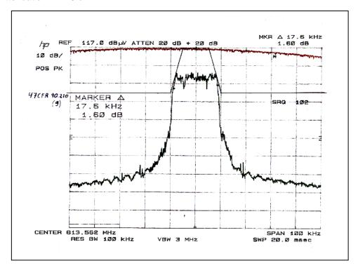
Spectrum Analyzer Plot: Emission Mask G: Tx @ 821 MHz Attenuation = 22.9 dB
