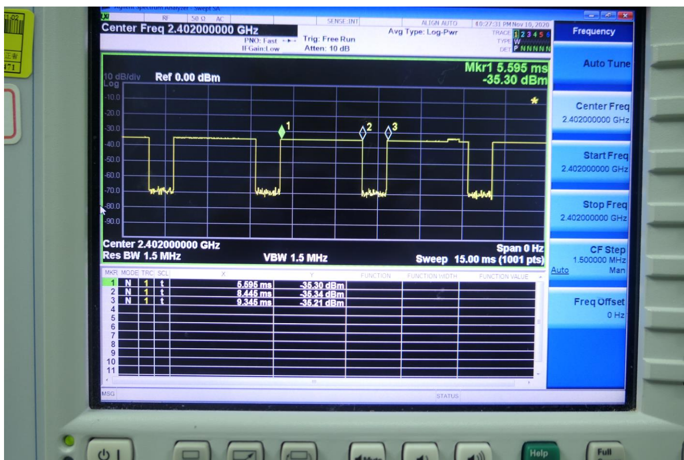
Time-domain plot for Bluetooth transmission signal
