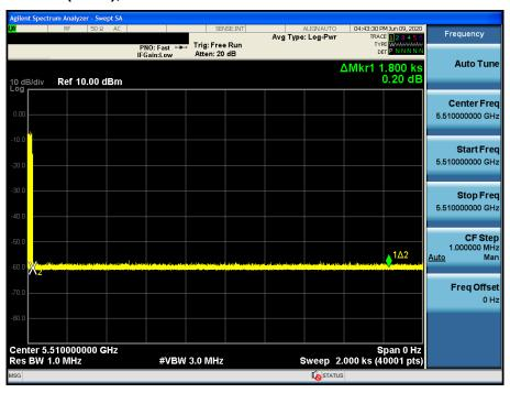
6.3. Radar simulation signal
