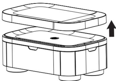
2. Push the upper cover of paper cassette as Figure 1 shown below, and then flip it to the back as Figure 2 shown below.
