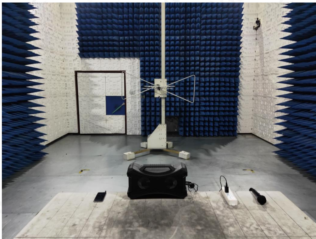
RADIATED EMISSION TEST SETUP ABOVE 1GHZ
