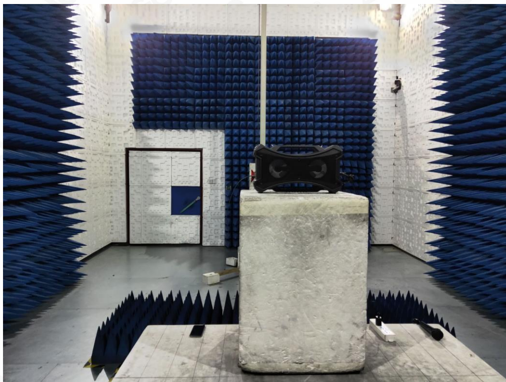
RADIATED EMISSION TEST SETUP ABOVE 1GHZ
