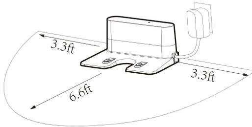
Place the charging base against the wall. Do not place any objects within 3.3 ft to the left / right and 6.6 ft to the front, and do not place any mirrors or other reflective objects within this distance.
