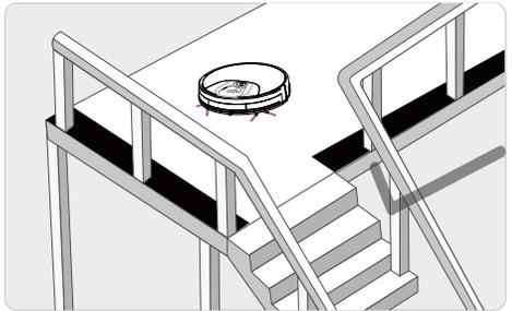
If the robot works at the stairway, the edge of the step, or the entrance to the narrow area among the furnitures, etc, please place a fence to ensure it is safe and running smoothly.
