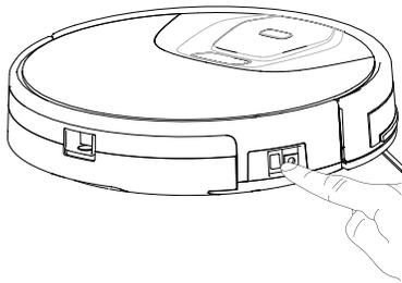
Switch on the robot, which makes the Control button green, and enter the Selected mode. If the robot is not activated within 10 minutes, the robot will enter Sleep mode.
