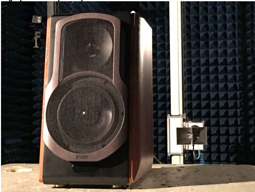
Photograph 4: Set-up for Spurious Emissions for 1 - 18GHz
