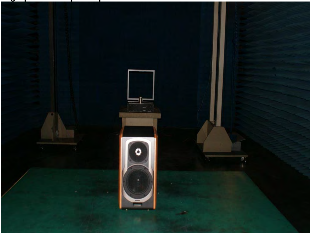
Photograph 2: Set-up for Spurious Emissions for below 30MHz
