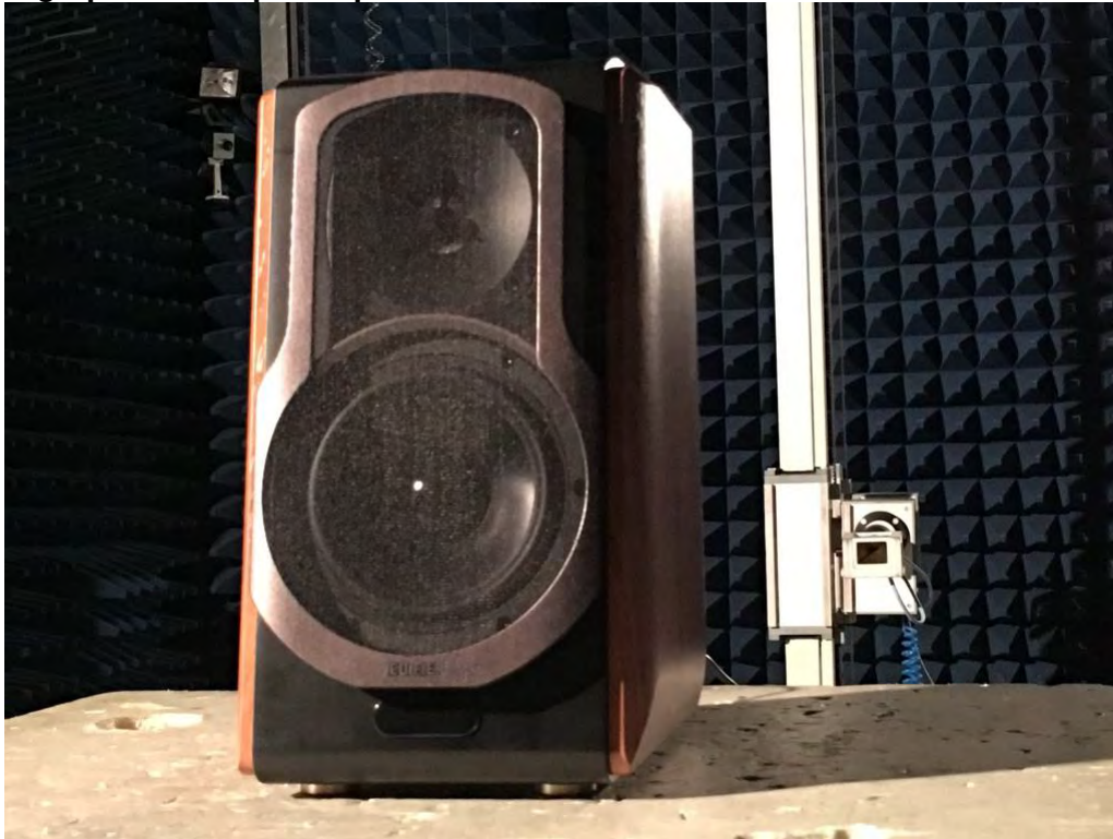
Photograph 5: Set-up for Spurious Emissions for 18 - 26.5GHz
