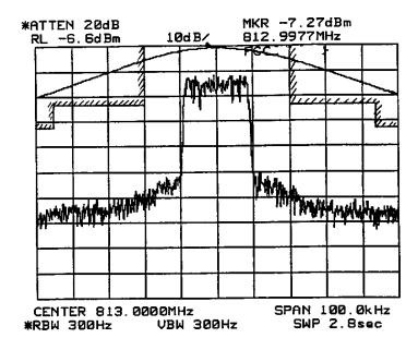
Occupied Bandwidth Test in Up-Link Transmission Mode.
