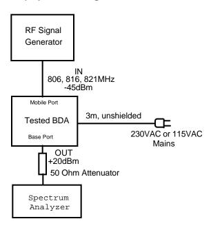
The tested equipment was conditioned with typical modulating signals to produce the worst case (i.e. the widest) bandwidth. In the case of MW-CBDA-ESMR-1W60 BDA 64kbits Per Second Pseudo-Random Digital Modulation was used.
