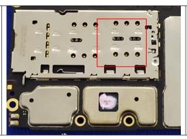
The PCB design of SIM2 remains, and the single-card version is implemented through physical card holders.
