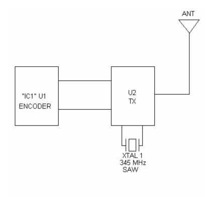
"IC1" (U1) is the Encoder ( 'Micro' )  $\,$  U2 is the single chip transmitter.
