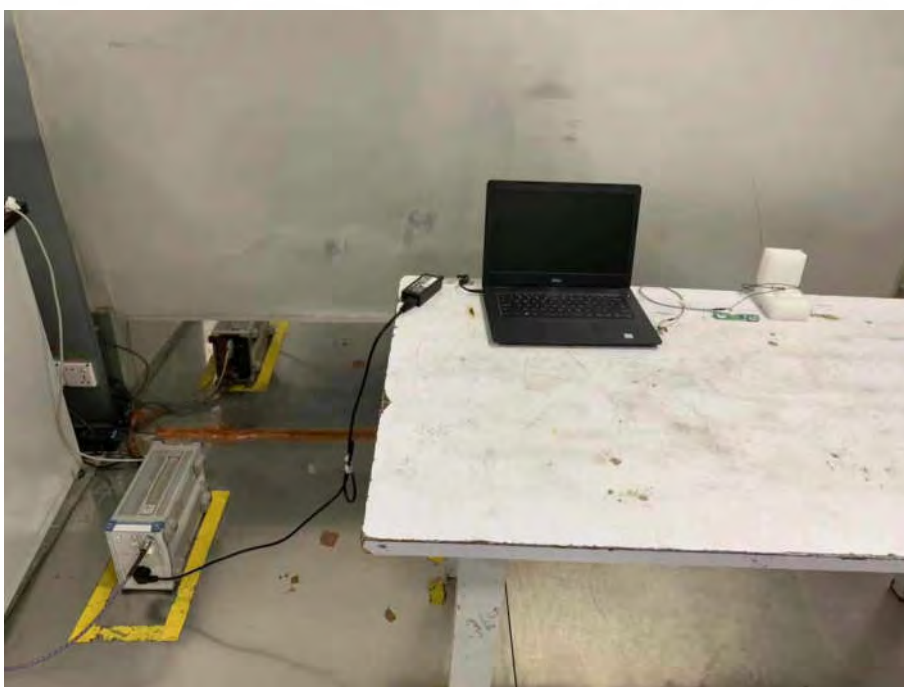
Conducted Emissions Test Setup
