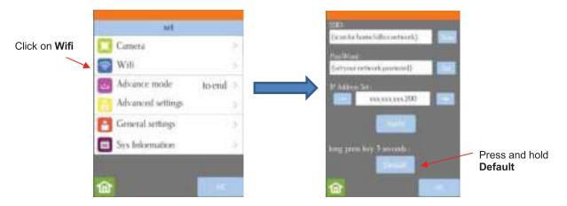
To reset the Skycut so that it will be found as an available network, press and hold the **Default** button for 3 seconds. Release and you should see the **Apply** button now displays **Wait**. In a minute the **Apply** should return and you can then proceed back to <u>A</u>. <u>The Skycut has never been set up wirelessly to a network</u> and use the same procedure as if the Skycut was never set up on a network.
