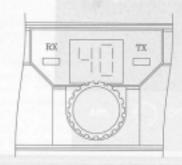
Step 7: To transmit, press the Push-totalk bar on the microphone. To receive, release the bar.
