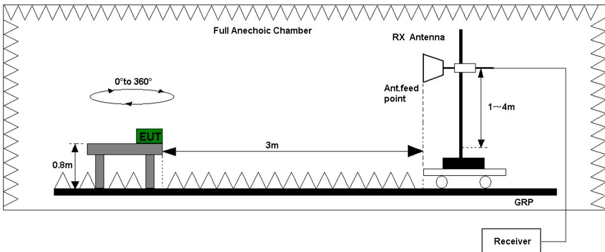
Figure 2. Test set-up of radiated disturbance(above 1GHz)
