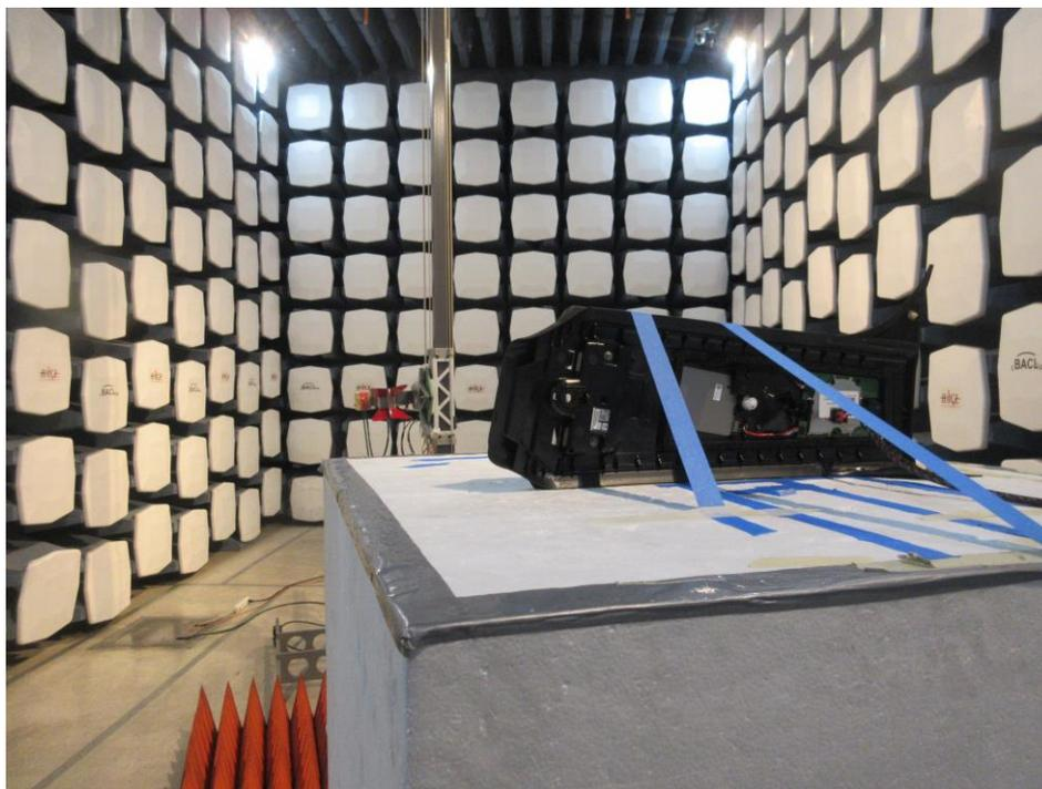
**1.7 Radiated Spurious Emissions measured at 1 meter, 18 GHz to 26.5 GHz, Front View**
