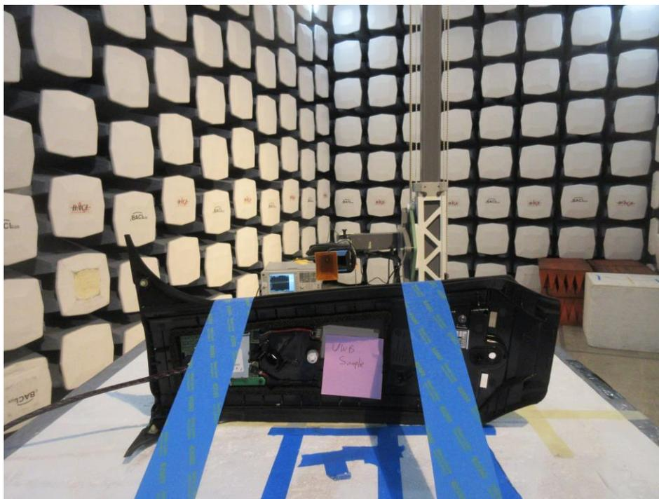
**1.9 Radiated Spurious Emissions measured at 1 meter, 26.5 GHz to 40 GHz, Front View**
