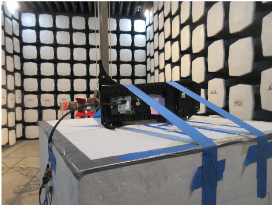
**1.5 Radiated Spurious Emissions measured at 3 meter, 1 GHz to 18 GHz, Front View**
