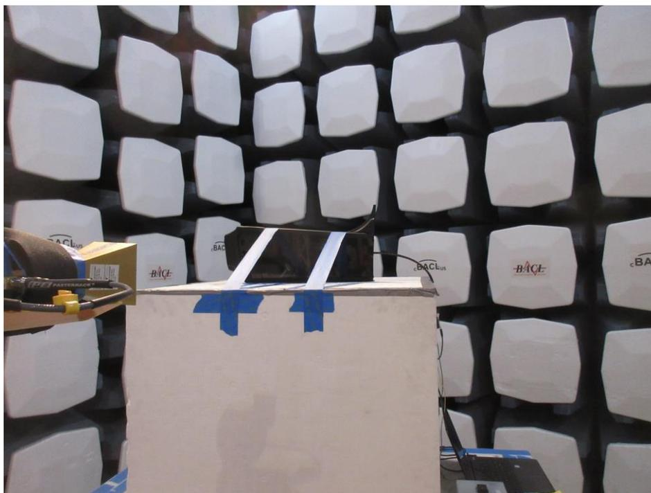
**1.10 Radiated Spurious Emissions measured at 1 meter, 26.5 GHz to 40 GHz, Rear View**
