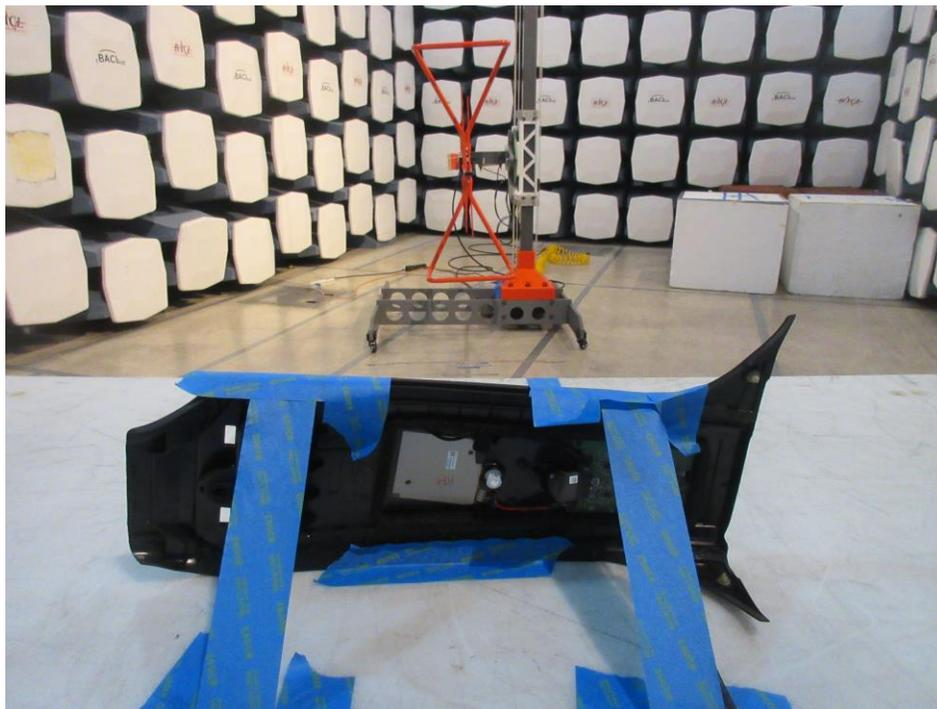
**1.3 Radiated Spurious Emissions measured at 1 meter, 1 GHz to 18 GHz, Front View**
