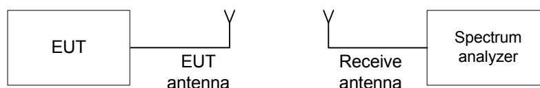
Figure 7.7.1 Band edge emission test setup
