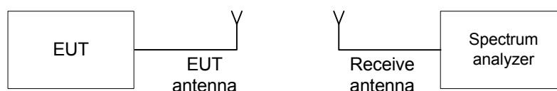
Figure 7.1.1 The 20 dB bandwidth test setup
