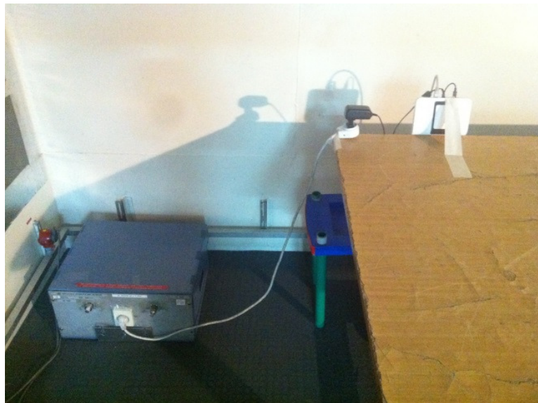
Photograph 8.1.1 Setup for conducted emission measurements
