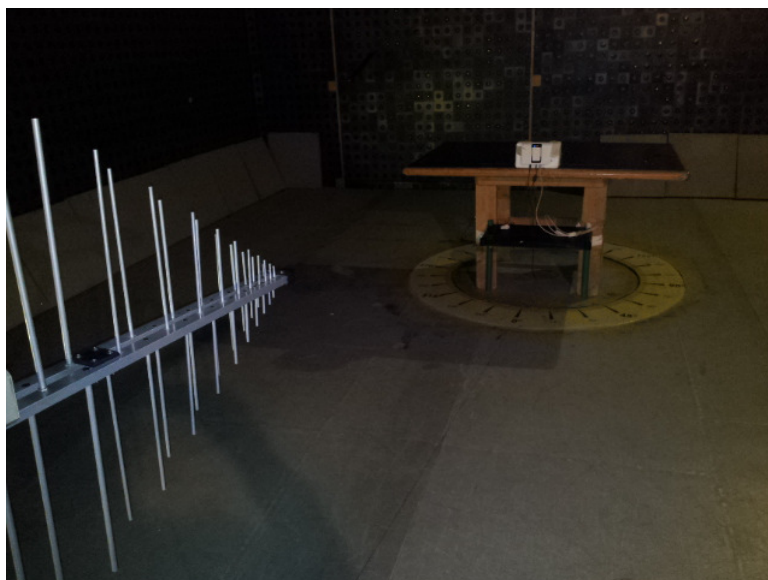
Photograph 8.2.2 Setup for radiated emission measurements, EUT cabling
