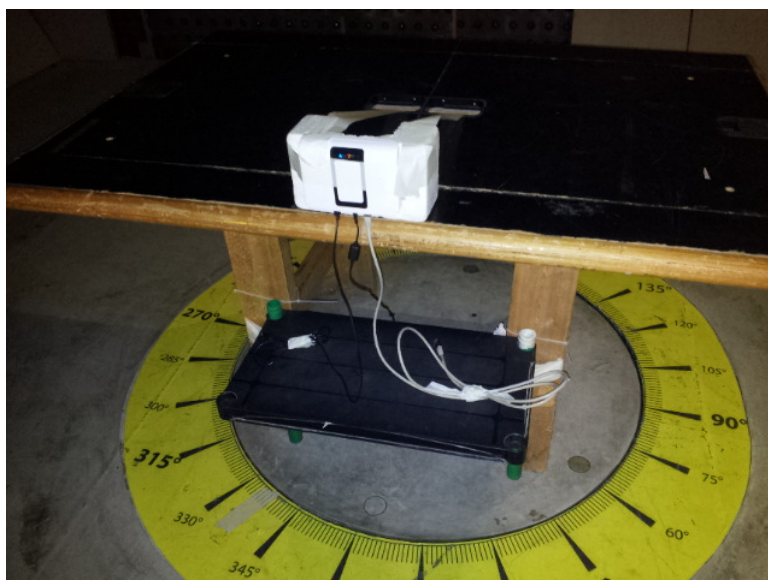
Photograph 8.2.2 Setup for radiated emission measurements, EUT cabling
