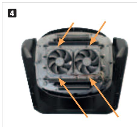
5. Use the two calibration screws to centre the hotspot (see markings).
