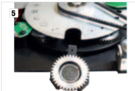
6. The gobo can now be removed from the bracket and replaced with another one.
