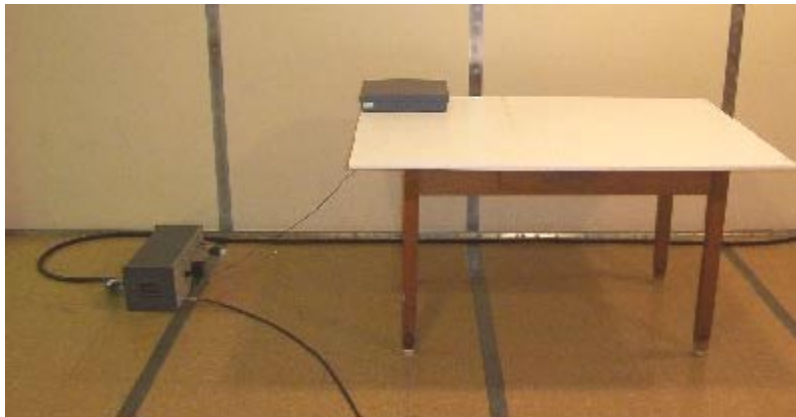
Staff Station Reader (Serial Version): Conducted Emission Test Setup
