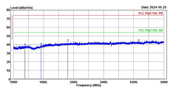
Condition : FCC Part 15C PK 3m EMCO\_3117\_82847 VERTICAL
