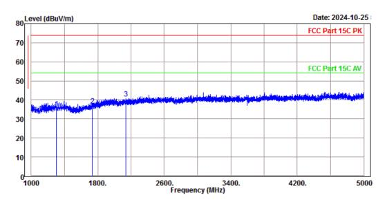
Condition : FCC Part 15C PK 3m EMCO\_3117\_82847 HORIZONTAL
