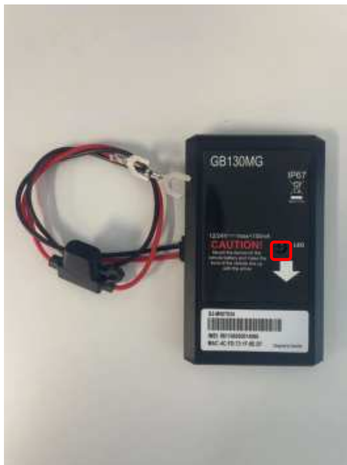
Figure 6. GB130MG LED on the Case
