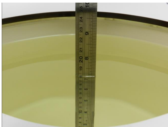
Fig 10.1 Photo of Liquid Height for Body SAR
