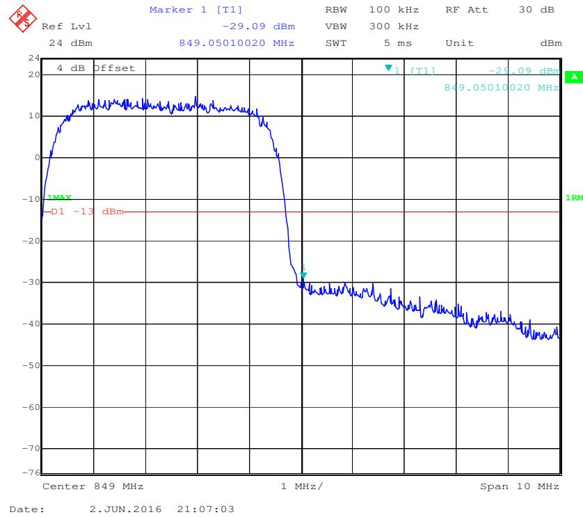
**Cellular Band, Left Band Edge for HSUPA (BPSK) Mode**
