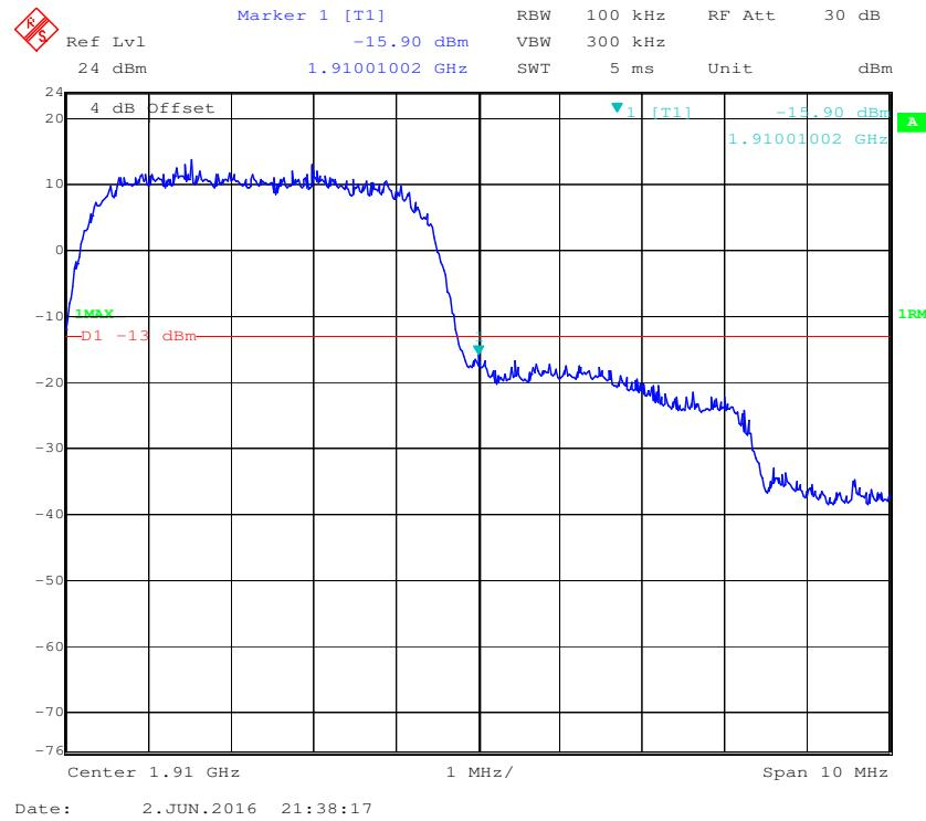
**PCS Band, Left Band Edge for HSDPA (16QAM) Mode**
