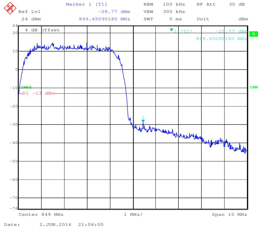
**PCS Band, Left Band Edge for GSM (GMSK) Mode**
