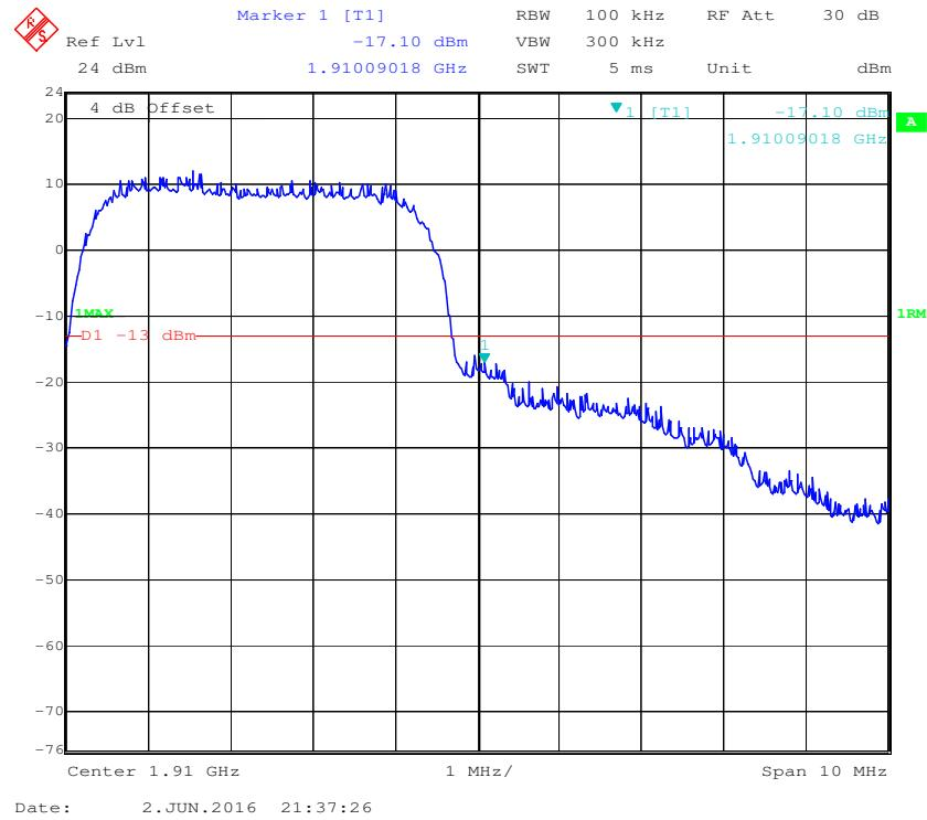
**PCS Band, Left Band Edge for HSUPA (BPSK) Mode**
