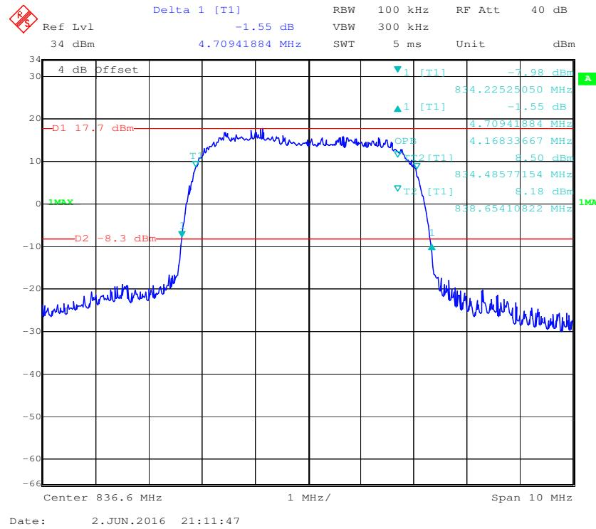
**PCS Band (Part 24E)****99%&26 dB Occupied Bandwidth for GSM (GMSK) Mode**
