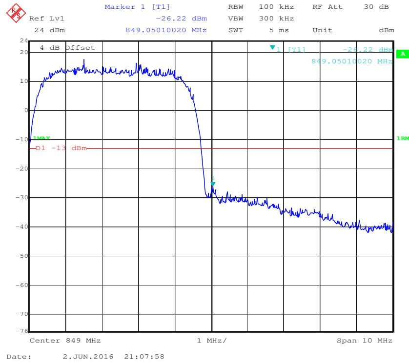
**Cellular Band, Left Band Edge for HSDPA (16QAM) Mode**
