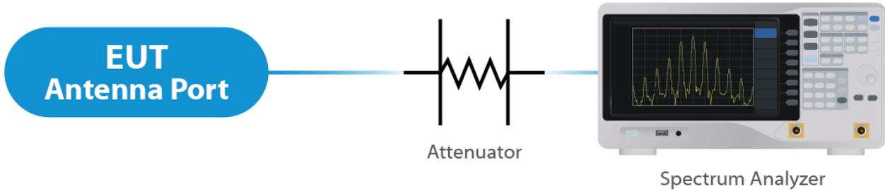
Figure 2: Direct Connect at the Antenna Port Test
