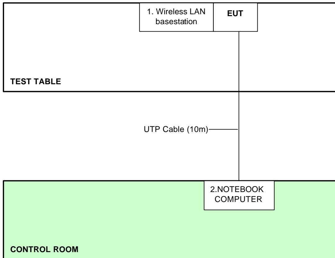
**NOTE:** 1. Support unit 2 was kept in the control room during the test.
