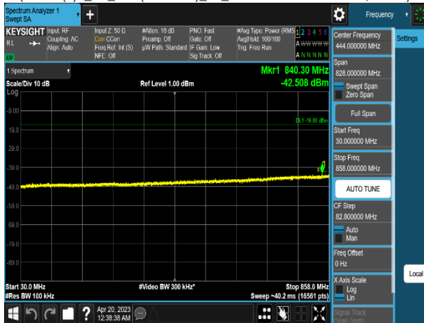
Plot 8-455. Conducted Spurious Emission Plot 30 MHz to 858 MHz (DSS B(n)5_1C_10M(5:5 Ratio)_2T_256QAM - Low Channel, Port 1)
