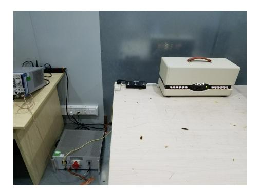
Radiation Emission Test Setup (Below 30MHz)
