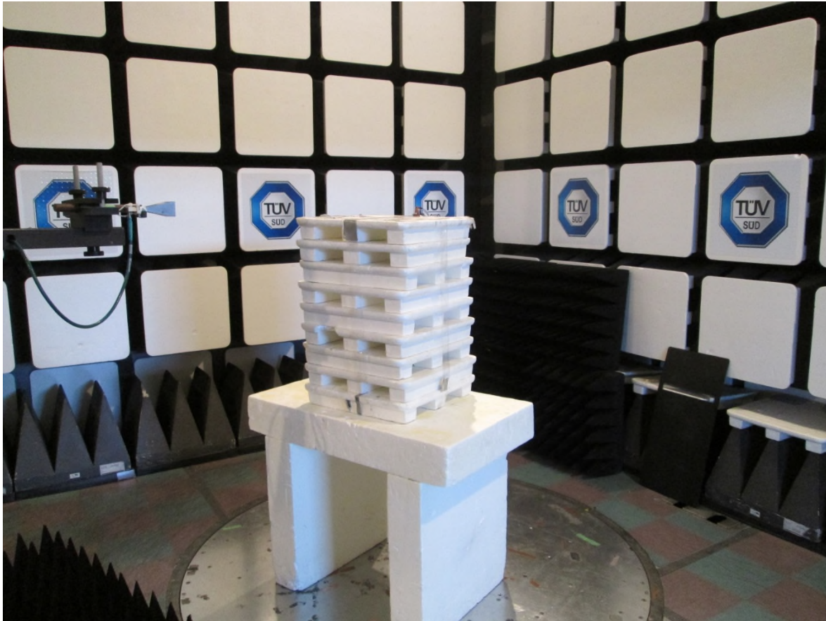
Figure 9 – Radiated Emissions Setup 18 GHz to 26.5 GHz
