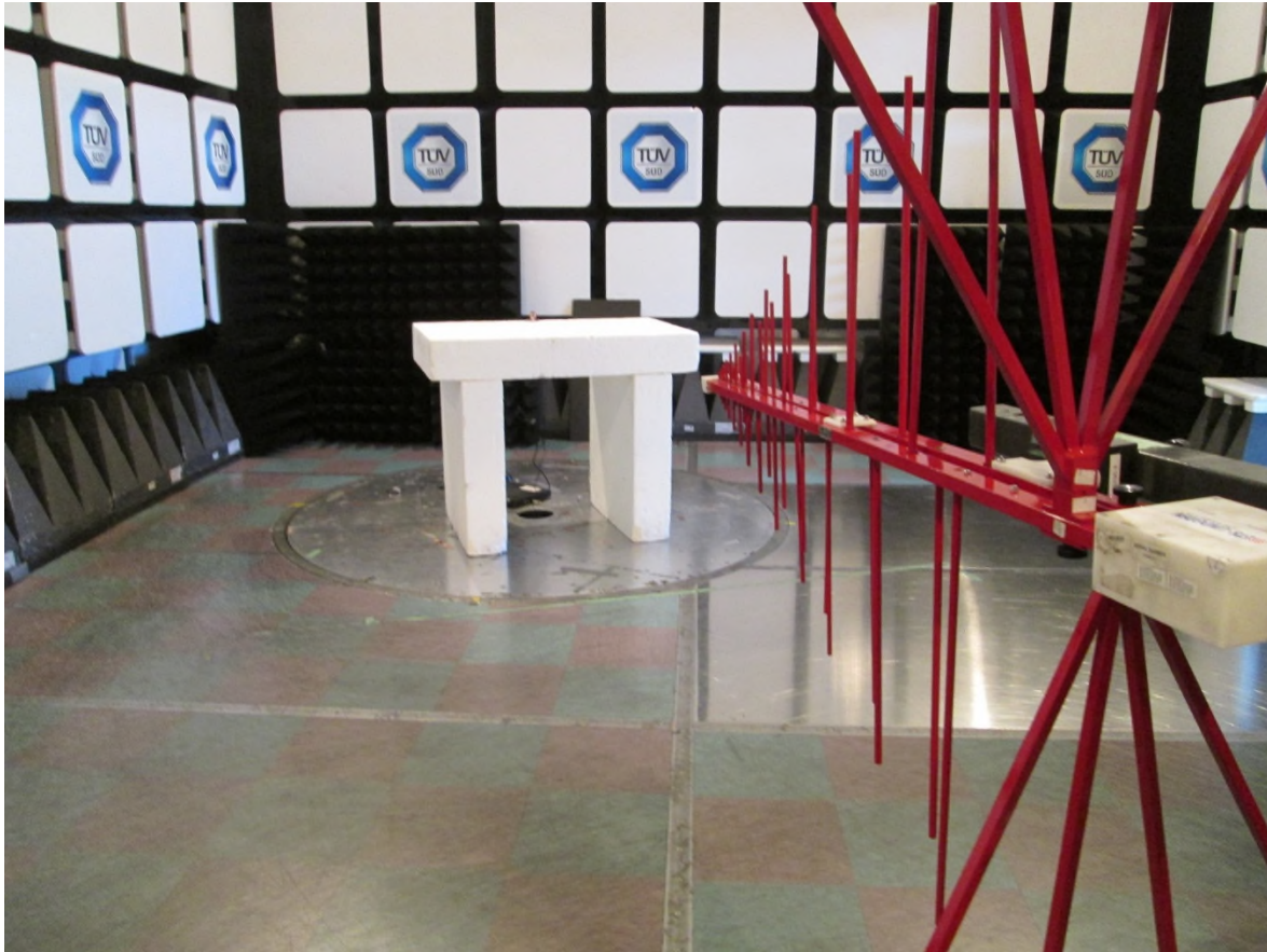
Figure 5 – Radiated Emissions Setup 30 MHz to 1 GHz
