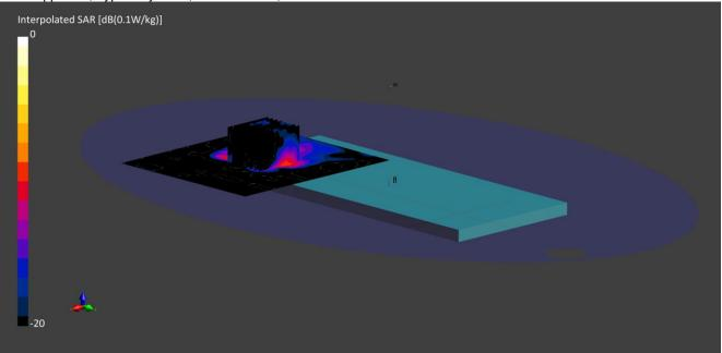
Communication System: IEEE 802.15.1 Bluetooth (GFSK, DH1) UID: 10030; Frequency: 2402.0 MHz; Duty Cycle: 0.31; Medium: HSL; Site61\_24Mar2021\_110352\_Head - 2450 5%; Medium parameters used: f = 2402.0 MHz;  $\sigma$  = 1.72 S/m;  $\epsilon_r$  = 39.6;  $\rho$  = 1000 kg/m3;  $\Delta\epsilon_r$  = 0.90 %;  $\Delta\sigma$  = -2.24 %; No correction Phantom section: Flat;
