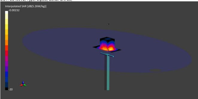
Communication System: CW UID: 0; Frequency: 2450.0 MHz; Duty Cycle: 1; Medium: HSL; Site61\_24Mar2021\_110352\_Head - 2450 5%; Medium parameters used: f = 2450.0 MHz;  $\sigma$  = 1.75 S/m;  $\epsilon_r$ = 39.6;  $\rho$  = 1000 kg/m3;  $\Delta \epsilon_r$ = 0.95 %;  $\Delta \sigma$  = -2.60 %; No correction Phantom section: Flat; DASY 6 Configuration:
